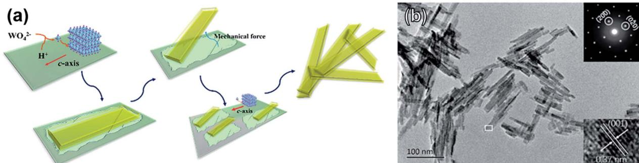
Fig. 6 (a) Schematic of  $\text{WO}_3 \cdot 2\text{H}_2\text{O}$  nanosheet formation through a solid-state mechanochemical reaction. (b) TEM image showing nanosheet morphology with inset selected-area diffraction pattern and lattice parameter measurement. Reprinted with permission from ref. 62, copyright 2017 American Chemical Society.
