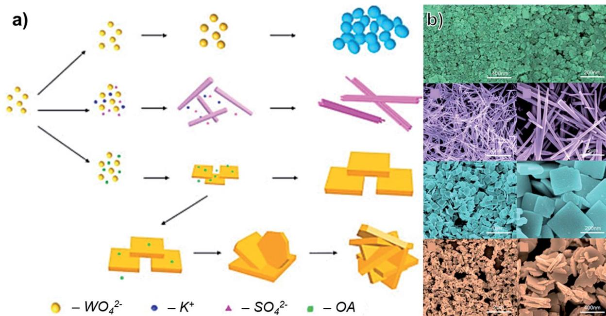
Fig. 2 (a) Schematic of different morphologies of WO<sub>3</sub> produced through a hydrothermal route with variation of precursors (OA: oxalic acid). (b) SEM images of the results structures at low and high magnification, adapted with permission from ref. 38, copyright 2016, Elsevier.
