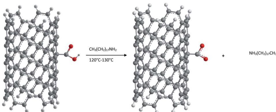
Fig. 8 Ionic functionalization of COOH functionalized CNTs.
