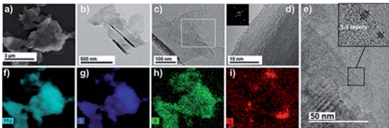
Fig. 9 SEM image (a) and EDS elemental maps of Mo, S, B and N (f-i), TEM and HRTEM images of the MoS<sub>2</sub>/h-BN hybrid (b-e).<sup>166</sup> Reprinted with permission from ref. 166 (Copyright © 2019, American Chemical Society).
