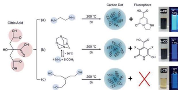
Fig. 14 Synthesis conditions of citric acid-based CDs using three different nitrogen-containing precursors. Figure reproduced from ref. 206 with permission from American Chemical Society, copyright 2017.
