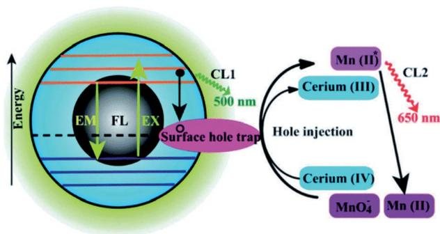
Fig. 20 Schematic illustration of the FL and CL mechanisms in the CDs-KMnO<sub>4</sub> and CDs-cerium(IV) systems. CL1 and CL2 represent two CL routes in the system. Figure reproduced from ref. 234 with permission from Royal Society of Chemistry, copyright 2012.
