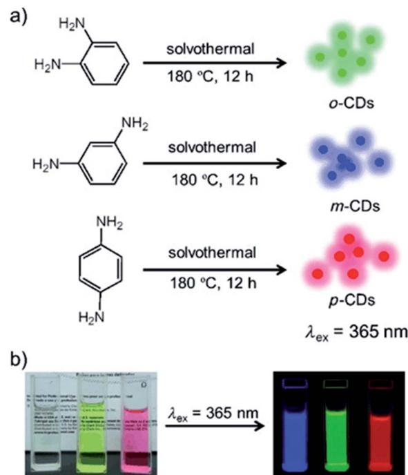
Fig. 6 (a) Preparation of the red, green and blue (RGB) PL CDs (CDs) from three different phenylenediamine isomers (*i.e.*, *o*-PD, *m*-PD and *p*-PD); (b) photographs of *m*-CDs, *o*-CDs, and *p*-CDs dispersed in ethanol in daylight (left), and under  $\lambda = 365$  nm UV irradiation (right). Figure adapted from ref. 160 with permission from Wiley, copyright 2015.
