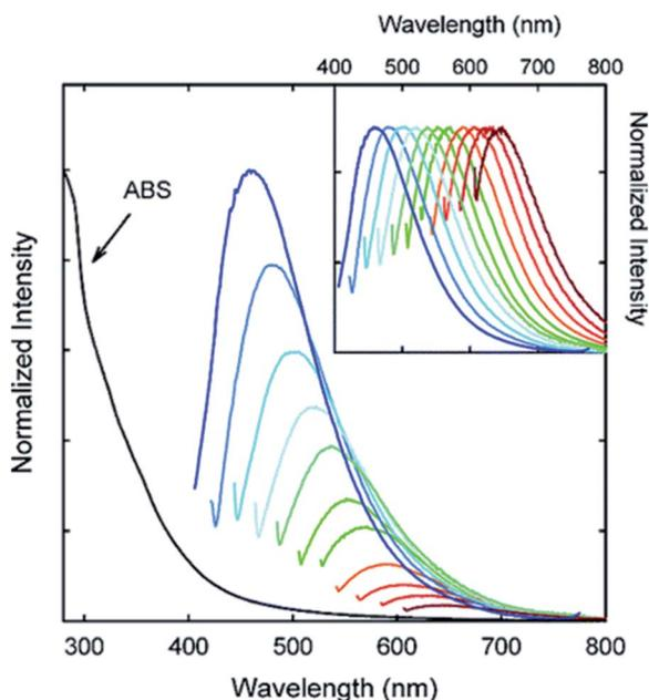
Fig. 10 Absorption and emission spectra of PPEI-EI passivated CDs in water with increasing  $\lambda_{\text{ex}}$  from 400 nm on the left with 20 nm increments. Inset: emission intensities normalized to quantum yields. Figure adapted from ref. 58 with permission from American Chemical Society, copyright 2006.
