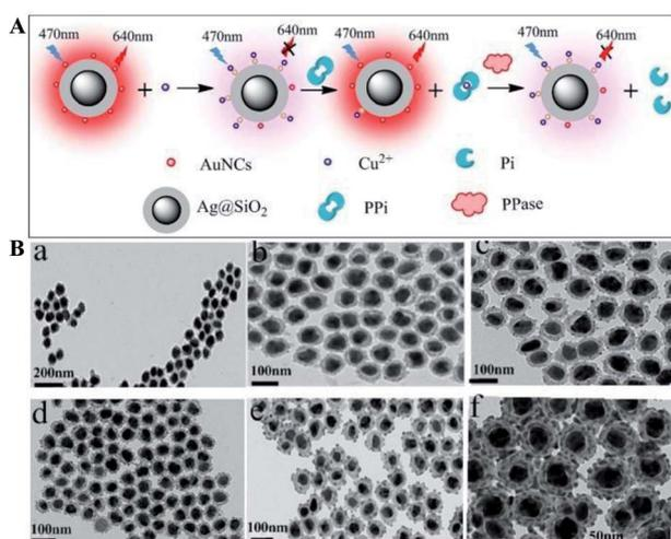
Fig. 3 (A) Schematic of sensing mechanisms of multiple components with Ag@SiO<sub>2</sub>-AuNCs, AuNCs refer to Au nanoclusters and (B) TEM micrographs of composite Ag@SiO<sub>2</sub> nanoparticles with different SiO<sub>2</sub> spacer thicknesses: (a) ~7 nm, (b) ~10 nm, (c) ~12 nm, (d) ~15 nm, (e) ~20 nm, and (f) ~25 nm. Reprinted from ref. 56 with permission.
