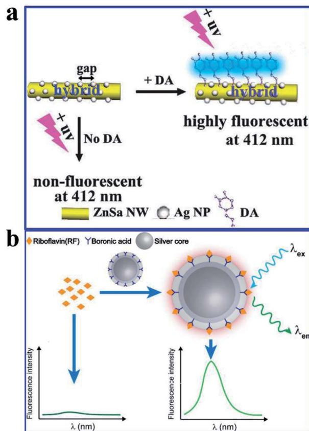
Fig. 17 (a) Schematic illustration of the hybrid that can improve DA fluorescence detection,  $\lambda_{em} = 350$  nm. Reproduced from ref. 51 with permission from the Royal Society of Chemistry. (b) Schematic showing the preparation processes and sensing mechanisms of the molecularly imprinted core-shell Ag@SiO<sub>2</sub> NPs for the fluorescence assay. Reprinted from ref. 99 with permission.
