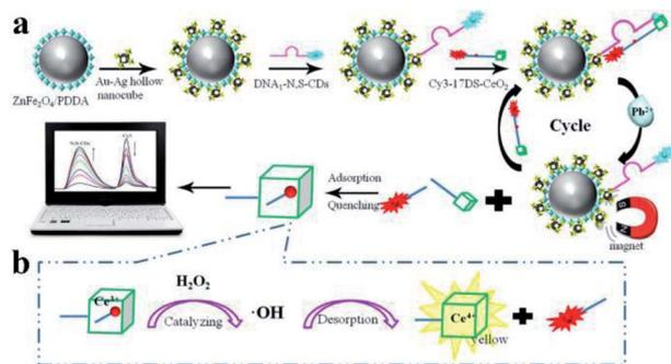
Fig. 6 Schematic showing the fabrication and sensing processes of the  $\text{Pb}^{2+}$  biosensor. Reprinted Scheme 1 with permission from Linlin Liang, Feifei Lan, Shenguang Ge, Jinghua Yu, Na Ren and Mei Yan, *Anal. Chem.*, 2017, **89**, 3597–3605 (ref. 158). Copyright 2017 American Chemical Society.
