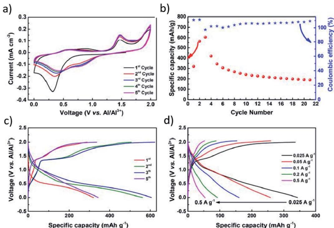
Fig. 7 Electrochemical performance of SPAN in Al-S battery applications. (a) Cyclic voltammograms, (b) cycle performance, (c) galvanostatic (dis-)charge curve, (d) rate capabilities.<sup>98</sup> Reproduced with permission. Copyright 2018 American Chemical Society.
