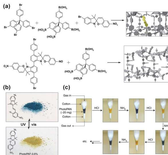
Fig. 26 (a) Structure of building blocks and monotopic and ditopic spiropyran pendants used to synthesize responsive porous organic polymers. (b) Light-induced changes in colour of the porous material bearing monotopic spiropyran photoswitch. (c) Changes in the colour of the material bearing ditopic spiropyran upon alternating protonation/deprotonation cycles of merocyanine pendants. Adapted by permission from Springer Nature from ref. 71, Copyright 2014.
