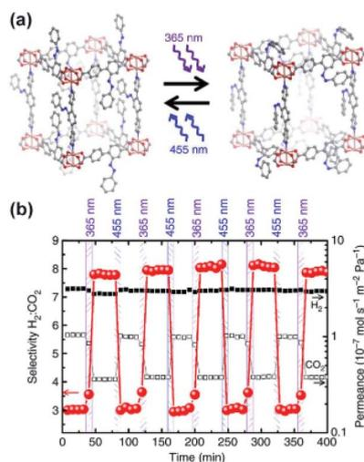
Fig. 11 (a) Representation of light induced structural changes in the SURMOF functionalized with azobenzene pendants. (b) Light-induced changes in selectivity of H<sub>2</sub>/CO<sub>2</sub> separation on  $\alpha$ -Al<sub>2</sub>O<sub>3</sub>-supported SURMOF membrane (red circles) and H<sub>2</sub> (black squares) and CO<sub>2</sub> (white squares). Adapted by permission from Springer Nature from ref. 126, Copyright 2014.
