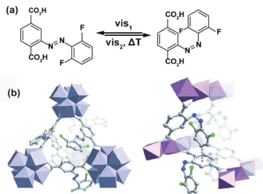
Fig. 9 (a) Structure and switching of the incorporated visible-light responsive *ortho*-fluoro azobenzene linker. Models of the solid-state structure of the isorecticular (b) UiO-66(Zr) (left panel) and MIL-53(Al) (right panel). Reprinted with permission from ref. 107. Copyright 2016 Wiley-VHC.
