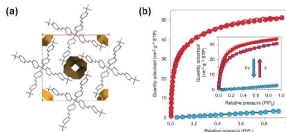
Fig. 12 (a) Packing of the tetrameric azobenzenes in the solid state along with representation of the empty channels. (b) CO<sub>2</sub> adsorption isotherms at 195 K of pristine material (red isotherm) and after exposure to UV light (blue isotherm). Reprinted by permission from Springer Nature from ref. 115, Copyright 2015.
