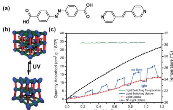
Fig. 8 (a) Structure of the stilbene bispyridyl pillar and azobenzene dicarboxylic acid used as linkers. (b) Depiction of the active framework. (c) Changes in the CO<sub>2</sub> adsorption isotherm of the material (black line, pristine), during *in situ* irradiation (red line) and upon a modulated exposure to light (blue line), temperature of the sample (green line). Reprinted with permission from ref. 106. Copyright 2013 Wiley-VHC.
