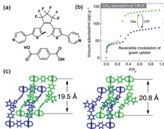
Fig. 15 (a) Structure of the linkers used to construct two-fold interpenetrated framework. (b)  $CO_2$  adsorption isotherms of pristine (green points) and irradiated (blue points) materials. (c) Representation of the SC X-ray structure of pristine (left) material and UV-treated (right) materials viewed along *b* direction. Adapted by permission from Springer Nature from ref. 121, Copyright 2017.
