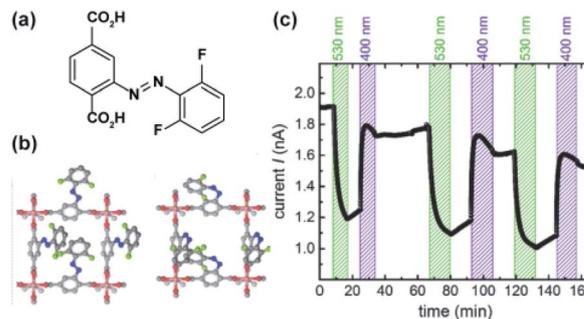
Fig. 23 (a) Structure of *ortho*-fluoro azobenzene linkers and (b) switchable SURMOF viewed in *c* direction. (c) Changes in the proton current conduction of butanediol in SURMOF at 1 V and 1 Hz upon alternating irradiation at 530 and 400 nm. Adapted with permission from ref. 145. Copyright 2018 Wiley-VHC.
