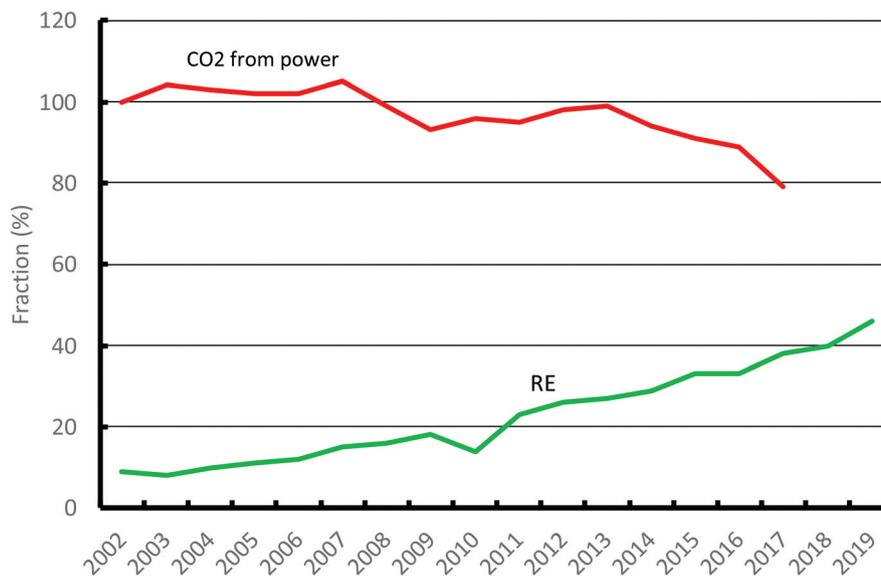
Fig. 2 Fractions of RE in the German power system (green) and change in power-related CO<sub>2</sub> emissions (red). The absolute CO<sub>2</sub> emission in 2002 was 372 Mt.
