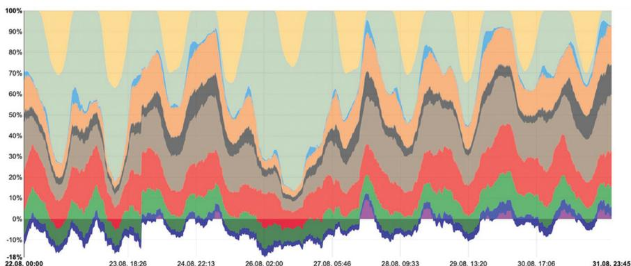
**Fig. 1** Energy mix of the German power grid throughout August 2020 in fractions of the total demand. The maximum power demand was 74 GW. The negative values represent the export, the purple elements the net import of power. Colour coding: yellow solar, light green wind, light blue pumped hydro, orange gas, dark brown coal, light brown lignite, red nuclear, green biomass, dark blue hydro. (Source: Fraunhofer ISE, Energy Charts.)
