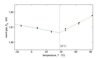
Fig. 5 Band gap (eV) (black dots) for perovskite composition  $Cs_{0.17}FA_{0.83}Pb(Br_{0.17}I_{0.83})_3$  as a function of temperature (°C), calculated from up and downward cycles of EQE, with a linear fit before discontinuity (blue dashed line) and after slope discontinuity (red dotted line). The grey dashed line shows the intersection of the two fit slopes.
