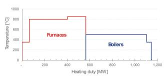
Fig. 4 Typical profile of energy demand of petrochemical plants (furnaces in red and boilers in blue).
