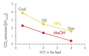
Fig. 6 Carbon intensity of fossil feedstocks for producing methanol and ammonia (adapted from Neelis<sup>68</sup>).
