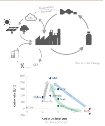
Fig. 8 Artist's impression of future sustainable carbo-chemical cycles (top) and shift in feedstock oxidation state (bottom; the carbon value has been defined as market price divided by carbon content, the carbon oxidation state has been calculated from the C:H:O ratio of the product following the eq. reported in the figure).
