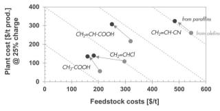
Fig. 3 Challenges in using natural gas. Top: thermodynamic limitation to yields in direct conversion of CH<sub>4</sub> (the acronyms are explained in the appendix).<sup>35</sup> Bottom: economic trade-off between feed and plant costs in direct oxidation of alkanes to chemical intermediates (black) vs. conventional olefin conversion (grey) (the diagonal dotted lines of the bottom figure represent the sum of feed cost and plant cost, the lion's share of the total manufacturing cost).36
