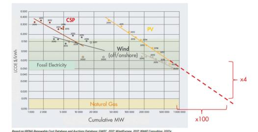
Fig. 5 Falling cost of renewable electricity and remaining cost gap with natural gas used as energy in industry (adapted from IRENA Renewable Power Generation Costs in 2017<sup>65</sup>).
