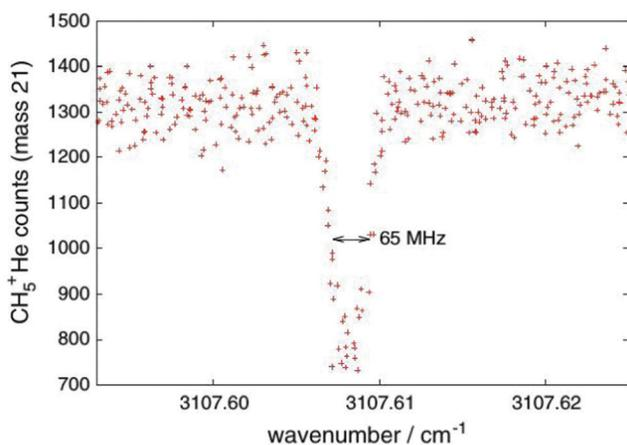
Fig. 4 First vibrational LIICG-signal, demonstrated for the floppy  $CH_5^+$  ion.<sup>42</sup> Reprinted with permission of Springer Nature.
