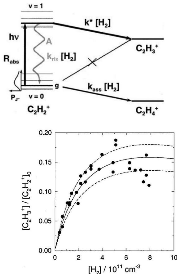
Fig. 3 (top) Level scheme for the LIR-process of  $\text{C}_2\text{H}_2^+$  showing all radiative and collisional rates. (bottom) LIR-signal for the  $P(9)$  transition as a function of the  $\text{H}_2$  number density, including three different solutions of the rate equation system.<sup>38</sup> Figures reprinted from ref. 38 with permission of AIP Publishing.
