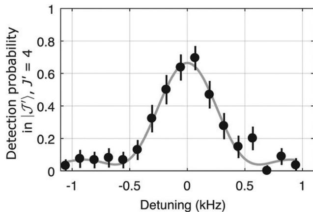
Fig. 19 After preparing a single  $^{40}\text{CaH}^+$  ion in the  $(J, m, \xi) = (2, -5/2, -)$  state, the probability to be in the  $(4, -7/2, -)$  state is detected by quantum-logic techniques.<sup>154,155</sup> When the comb Raman pulses (duration 1.6 ms) drive the transition  $(4, -7/2, -) \leftarrow (2, -5/2, -)$  at a difference frequency 1.992911000121(16) THz, the  $^{40}\text{CaH}^+$  ion is coherently transferred into this state. Figure reprinted from ref. 155 with permission of AAAS.
