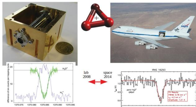
Fig. 7 (Left) Action spectrum of the  $\text{H}_2\text{D}^+$  rotational transition  $1_{01} \leftarrow 0_{00}$  (blue arrow in Fig. 5), observed as a decrease of the  $\text{H}_2\text{D}^+$  parent species and a simultaneous increase of the  $\text{H}_3^+$  product ion counts when the excitation frequency is in resonance.<sup>45</sup> (right) Detection of this transition towards IRAS 16 293 with the airborne far-infrared observatory SOFIA.<sup>88</sup>
