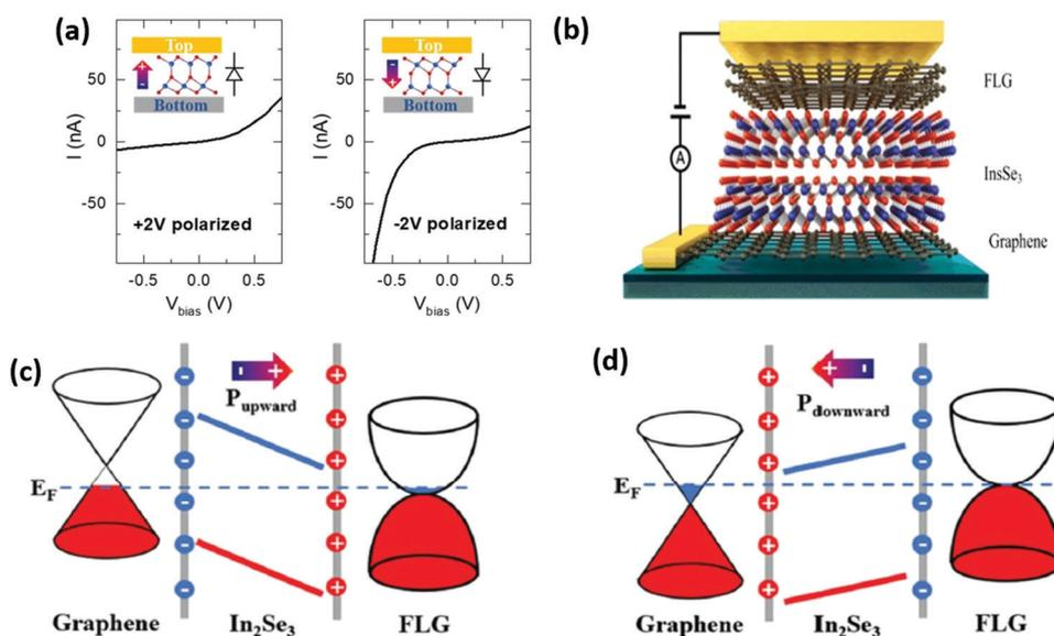
Fig. 3 (a) Schematic diagram of ferroelectric adjustable diode structure. (b)  $I$ - $V$  curve of diode rectification function. (c and d) Explanation of the switchable rectification behaviour of a ferroelectric diode, showing the energy band diagram of the graphene/ $\text{In}_2\text{Se}_3$  heterostructure and the evolution of the Schottky barrier in the ferroelectric polarization reversal. (Reproduced from ref. 40 with permission from The Royal Society of Chemistry.)
