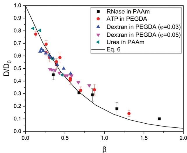
**Fig. 3** Relative diffusivity corresponding to real gel/solute systems as a function of  $\beta = \varphi(1 + R_s/R_m)^{1.3}$ . The prediction obtained from eqn (6) is also plotted (solid line). These diffusivities (and their error bars) were extracted from ref. 32,36,37,38.
