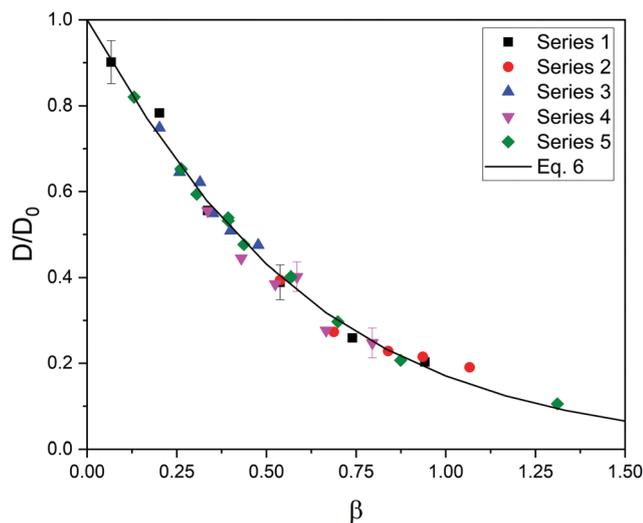
**Fig. 2** Relative diffusivity corresponding to five series of data as a function of  $\beta = \varphi(1 + R_s/R_m)^{1.3}$ . The best fit obtained from eqn (6) is also plotted (solid line). The error bars of a few cases are shown to exemplify the uncertainty in the relative diffusivity.
