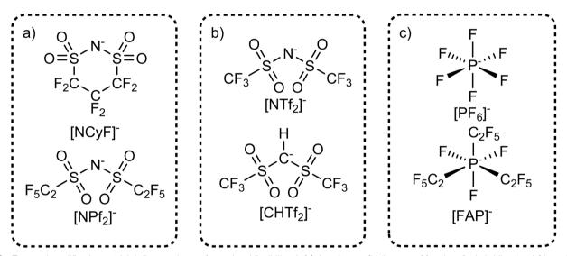
Fig. 10 Targeted modifications which influence the conformational flexibility via (a) ring closure, (b) degrees of freedom for hybridization, (c) introducing flexible groups.
