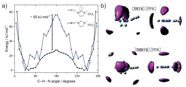
Fig. 20 (a) Energy as a function of the angle between C2 carbon, acidic hydrogen, and imide-N of the  $[NTf_2]$ . (b) Spatial distribution function of  $[PF_6]$  around  $[C_4C_1im]$  (top) and  $[C_4C_1im]$  (bottom). Reproduced from ref. 257 with permission from the PCCP Owner Societies.
