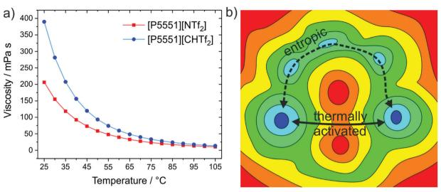
Fig. 12 (a) The ionic liquid with the more rigid anion, [P5551][CHTf<sub>2</sub>], has an almost twofold viscosity at room temperature compared to the ionic liquid with flexible anion, [P5551][NTf<sub>2</sub>]. <sup>140</sup> (b) The viscosity difference decreases with increasing temperature, which can be explained with basin theory, as more and more pathways become thermally activated. <sup>180,378</sup>
