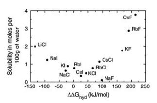
**Fig. 4** The solubility of simple alkali halides in water can be rationalised with size differences. Reprinted from J. Gujt, M. Bešter-Rogač and B. Hribar-Lee, *J. Mol. Liq.*, **190**, 34–41, Copyright 2014, with permission from Elsevier.
