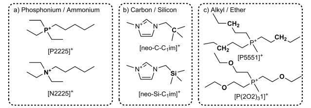
Fig. 7 Isostructural cation analogues serve as a targeted modification to probe the effects of conformation and conformational flexibility. All ionic liquids have  $[NTf_2]^-$  as anion.  $^{138,140,143}$
