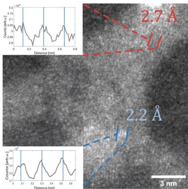
Fig. 17 STEM HAADF image of a  $V_2O_5$  particle (synthesised at 5.4 K cold head temperature). Two regions are marked where lattice constants could be extracted from the image. The respective intensity profile between the lines is shown in the inset. The black lines indicate a group of planes with a spacing of 2.7 Å the blue lines mark a group of planes with a spacing of 2.2 Å. Ref. 128 – reprinted with permission of the PCCP Owner Societies.
