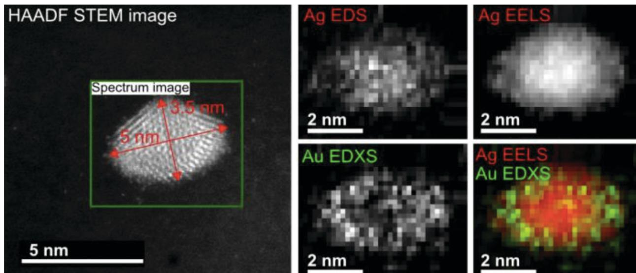
Fig. 13 EELS and EDXS elemental maps of an Ag@Au core@shell nanocluster acquired at a tilt angle of  $65^\circ$ . The boxed region in the HAADF STEM image indicates the area of the mapped region and the size of the cluster. The maps have been generated from the EDXS signal of the Ag and Au L-lines, and for the EELS signal the Ag M-edge intensity was extracted. The color overlay was formed from the Ag EELS and the Au EDXS signal. Reprinted from ref. 78 under the Creative Commons License.
