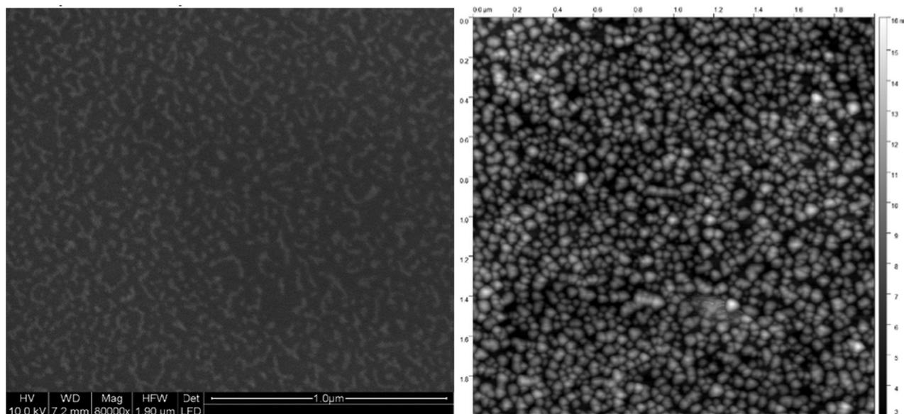
Fig. 6 Ag@Au core@shell nanoparticles of elongated shape, similar to ref. 60, imaged with an ESEM at only 10 nm resolution (left panel) compared to an AFM image in the tapping mode with an undetermined tip size (right panel). The scale is the same with the total area being  $2 \mu\text{m} \times 2 \mu\text{m}$ . The coverage is estimated as 26% based on the ESEM image while the AFM gives the impression of a higher coverage.<sup>60</sup>
