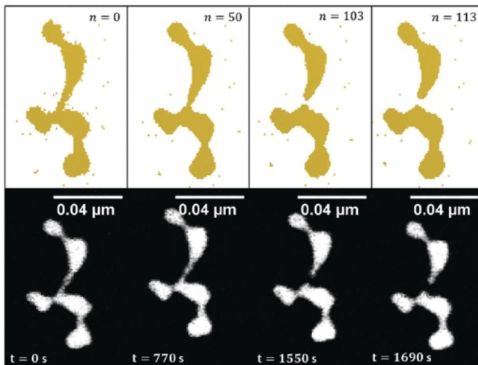
Fig. 11 Time evolved surface diffusion process of a gold nanowire at 150 °C. The observed *in situ* breakup event is studied over a time period of nearly half an hour (lower images) and are compared to the results obtained with the CA (upper images) in order to draw a fit between iteration steps and experimental observation time. Ref. 101 – reprinted with permission of the PCCP Owner Societies.
