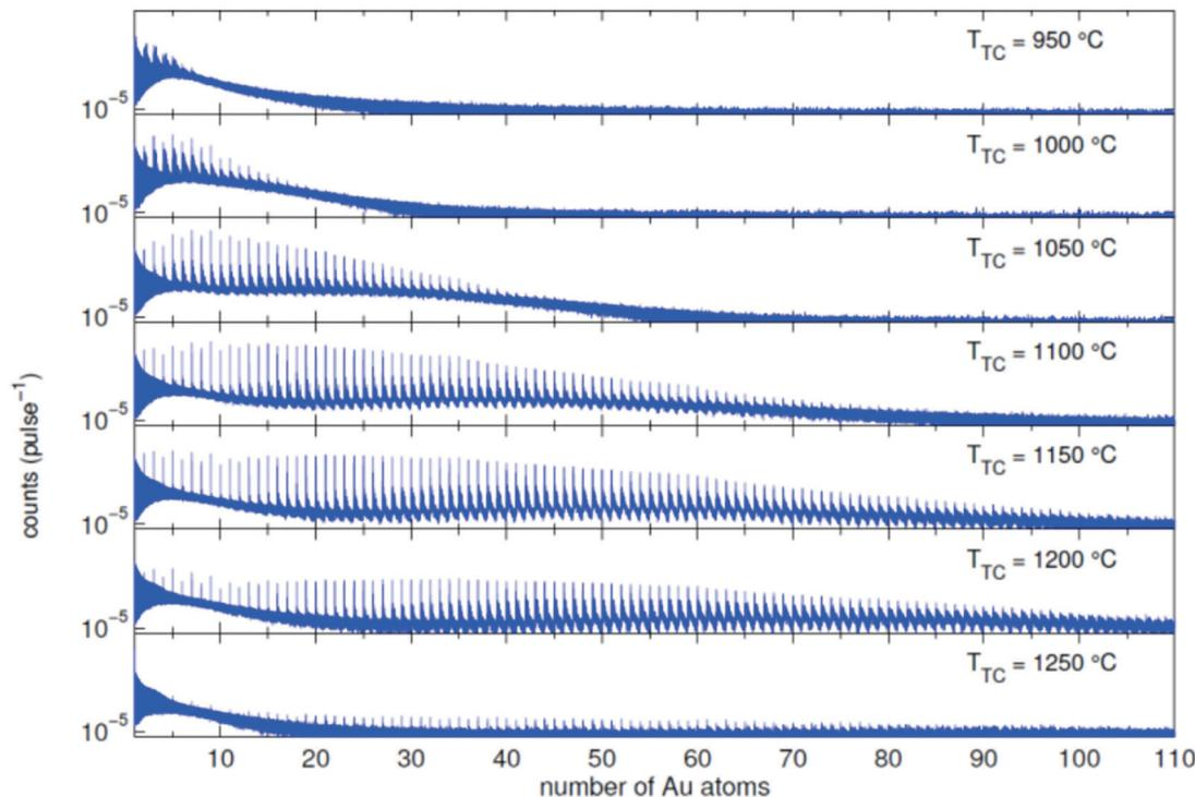
Fig. 2 Mass spectra of an Au doped He droplet beam ( $T_0 = 9$  K and  $p_0 = 20$  bar,  $N_{\text{He}} \approx 1.8 \times 10^6$ ) for different oven temperatures  $T_{\text{TC}}$ . Additional peaks appear due to the adsorption of water molecules in the pickup chamber.<sup>70</sup>
