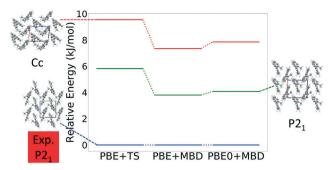
Fig. 22 Reranking of 4,5-dimethylphenanthrene structures generated by GAtor using increasingly accurate DFT functionals and dispersion methods. Relative energies are referenced to the lowest energy structure with each method. The experimental structure and two of the low energy putative structures are shown with the a, b, and c lattice vectors colored in red, green, and blue, respectively.
