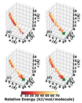
**Fig.** 21 Lattice parameter distributions of the 4,5-dimethylphenanthrene structures generated in GAtor runs using the energy-based fitness function with crossover probabilities of (a) 25% and (b) 75% and the niching fitness function with crossover probabilities of (c) 25% and (d) 75%. Structures are colored according to their relative energy, with darker colors corresponding to lower relative energies. If found, the experimental structure is indicated by a green X.
