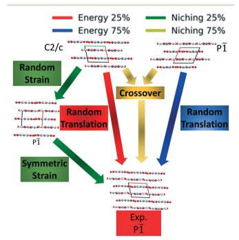
Fig. 5 The evolutionary routes that produced the experimental structure of TATB in different GA runs. The packing motifs and space groups of all structures are also shown. The a, b, and c axes are colored in red, green, and blue, respectively.
