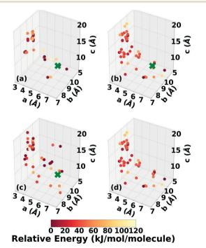
Fig. 3 Lattice parameter distributions of relaxed structures of TATB produced by Genarris runs using  $s_r$  values of (a) 0.85, (b) 0.75, and (c) 0.65. (d) The combined initial pool comprising 65 unique structures. Structures are colored according to their relative energy, with darker colors corresponding to lower relative energies. If present, the experimental structure is indicated by a green X.
