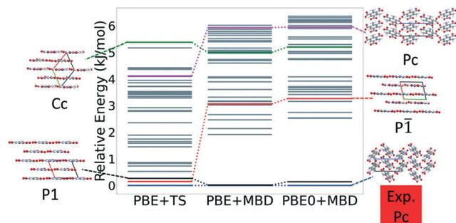
**Fig. 13** Reranking of DATB structures generated by GAtor using increasingly accurate DFT functionals and dispersion methods. Relative energies are referenced to the lowest energy structure with each method. The experimental structure and some low energy structures are shown with the *a*, *b*, and *c* lattice vectors colored in red, green, and blue, respectively.
