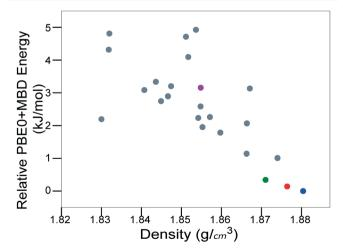
Fig. 8 PBEO + MBD relative energy as a function of density for TATB structures produced by GAtor. Colored markers correspond to structures shown in the same colors in Fig. 7.
