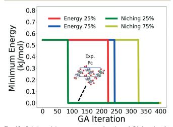
Fig. 10 Relative minimum energy as a function of GA iteration for DATB. The packing motif of the experimental structure, which is the minimum energy structure, is shown. The a, b, and c axes are colored in red, green, and blue, respectively.
