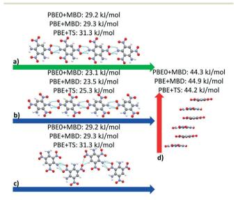
Fig. 14 Interaction chain analysis for the structures colored in (a and b) red, (c) purple, and (d) green in Fig. 13. The interactions are shown along the respective lattice vectors, with the a, b, and c lattice vectors colored in red, green, and blue, respectively. Hydrogen bonds are shown in light blue.
