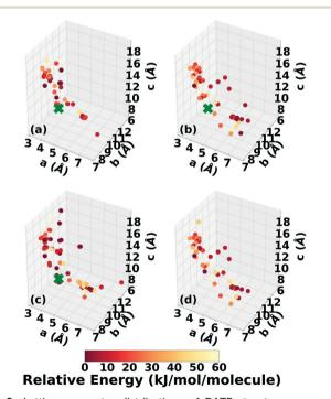
Fig. 9 Lattice parameter distributions of DATB structures generated by Genarris using  $s_r$  values of (a) 0.85, (b) 0.75, and (c) 0.65. (d) The combined initial pool comprising 65 unique structures. The structures are colored according to their relative energy, with darker colors corresponding to lower relative energies. If generated, the experimental structure is indicated by a green X.
