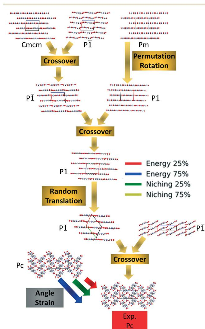
Fig. 11 Evolutionary routes that produced the experimental structure of DATB in different GA runs. The packing motifs and space groups of all structures are shown. The *a*, *b*, and *c* axes are colored in red, green, and blue, respectively.
