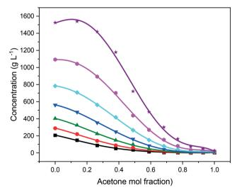
Fig. 5 Solubility of eicosane in toluene: acetone mixtures at different temperatures: 10 °C (black squares), 12.5 °C (red circles), 15 °C (green upward-triangles), 17.5 °C (blue downward-triangles), 20 °C (cyan diamonds), 22.5 °C (pink hexagons) and 25 °C (purple stars).
