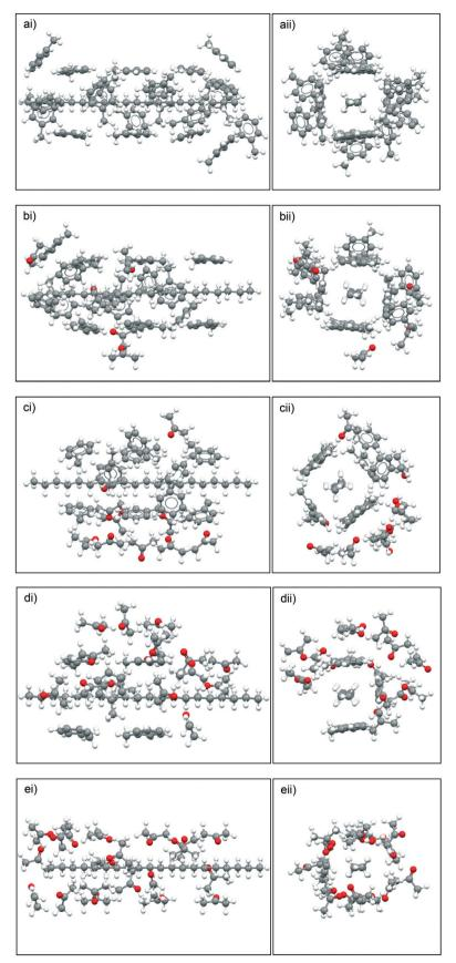
Fig. 10 Solvent clusters built using the intermolecular grid-search method around eicosane molecules, in different toluene: acetone ratios, with toluene molecule interactions determined first, followed by acetone molecules. a) 20:0; b) 15:5; c) 10:10; d) 5:15 and e) 0:20. i) and ii) represent different views of solvation clusters along and down the carbon backbone of eicosane, respectively.
