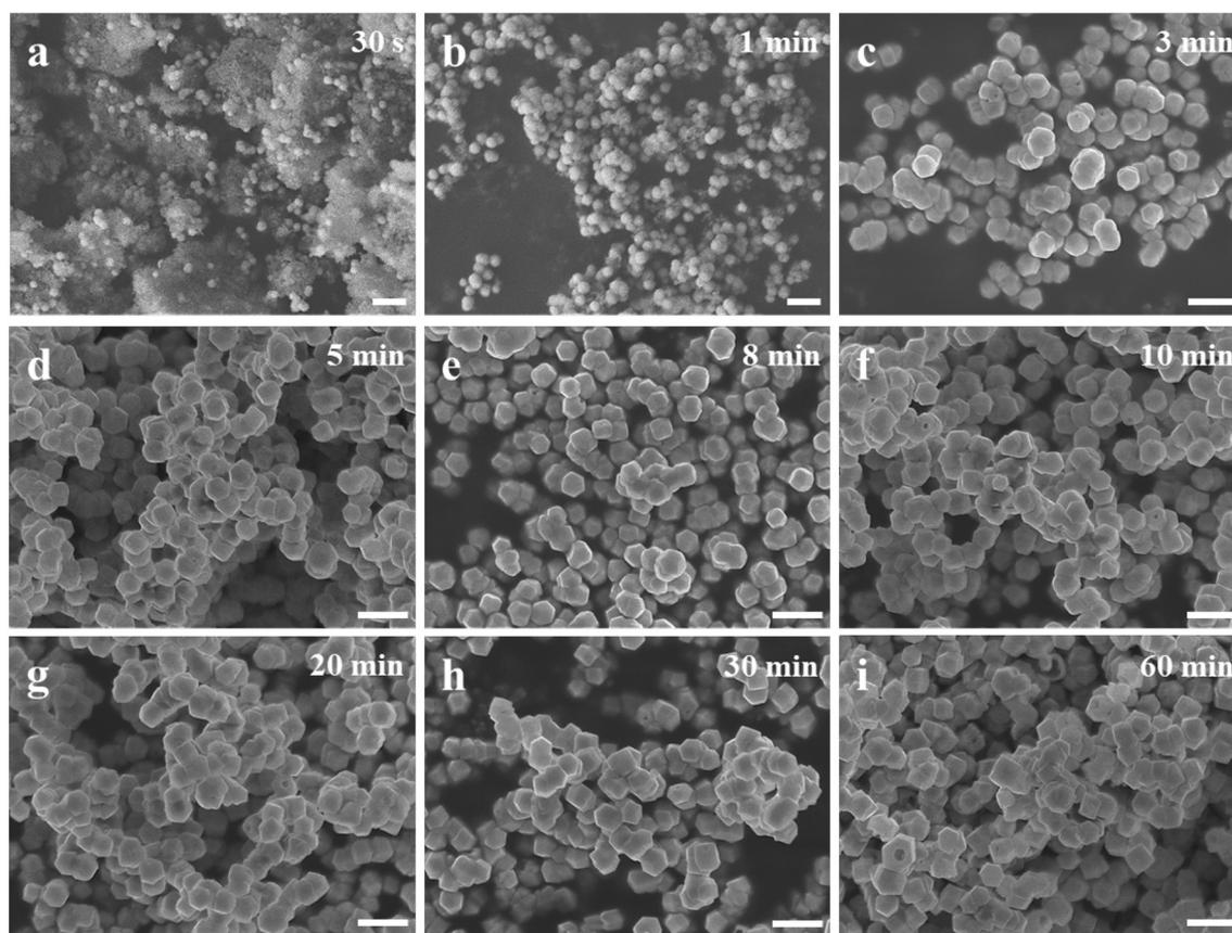
Fig. 2 SEM images of d-Cu<sub>2</sub>O nanoparticles synthesized using a 40 °C water bath with different reaction times: (a) 30 s, (b) 1 min, (c) 3 min, (d) 5 min, (e) 8 min, (f) 10 min, (g) 20 min, (h) 30 min and (i) 60 min. Scale bars = 500 nm.
