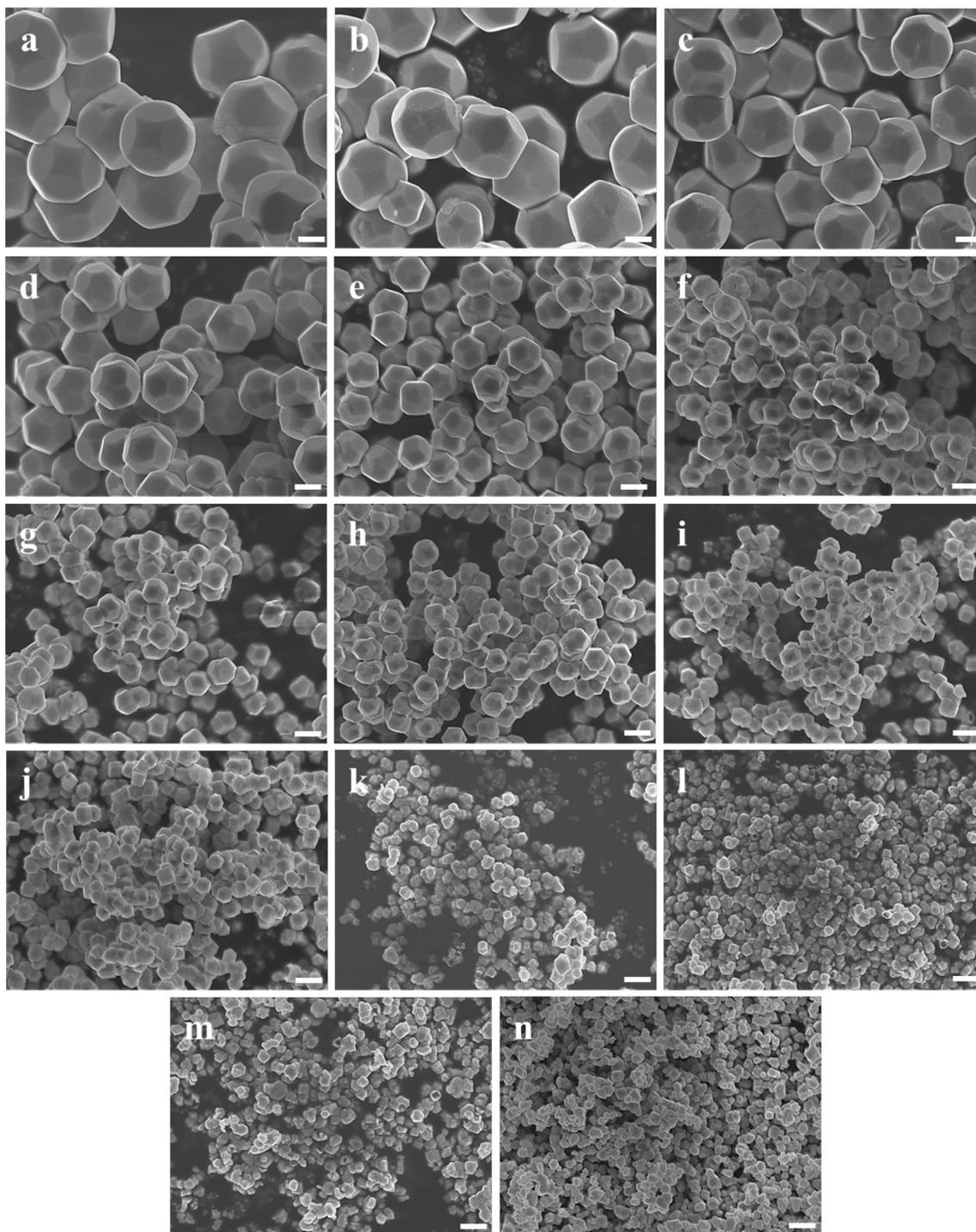
**Fig. 5** SEM images of d-Cu<sub>2</sub>O synthesized at different temperatures: (a) 31 °C, (b) 32 °C, (c) 33 °C, (d) 34 °C, (e) 35 °C, (f) 36 °C, (g) 37 °C, (h) 38 °C, (i) 39 °C, (j) 40 °C, (k) 45 °C, (l) 50 °C, (m) 55 °C and (n) 60 °C. Scale bars = 500 nm.
