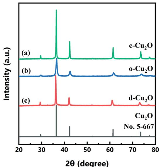
Fig. 6 XRD patterns of (a) c-Cu<sub>2</sub>O, (b) o-Cu<sub>2</sub>O and (c) d-Cu<sub>2</sub>O (synthesized at 40 °C). The XRD pattern of standard card of Cu<sub>2</sub>O (JCPDS 5-667) is also shown.
