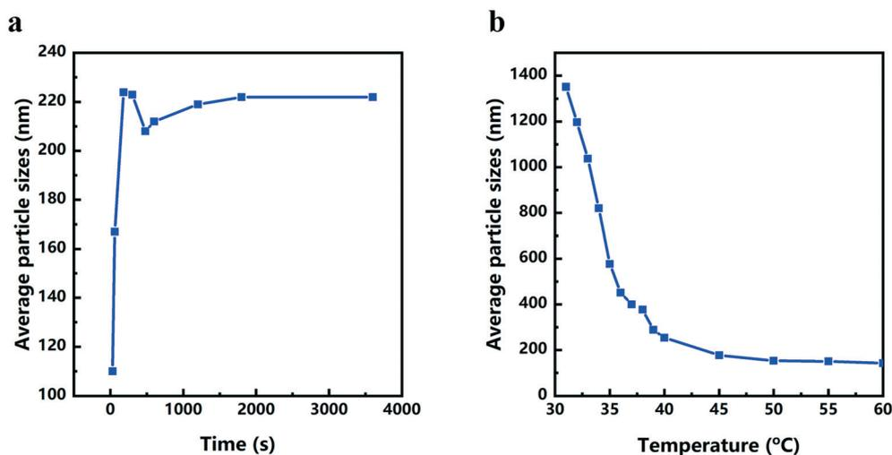
Fig. 4 (a) Reaction time dependence of average particle size of d-Cu<sub>2</sub>O obtained at a synthesis temperature of 40 °C. (b) Reaction temperature dependence of the average particle size of d-Cu<sub>2</sub>O after reaction of 1 h.
