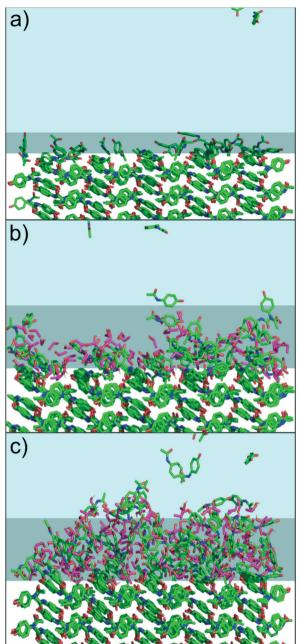
Fig. 4 Snapshots of molecular dynamics (MD) simulations of paracetamol (green) exposed to a) 0% ethanol (pink), b) 20%, and c) 40% ethanol-water mixture. In b) and c), a dynamic heterogeneous disordered surface (DHDS) layer has formed in the solid-solution interface. Stable crystal surface layer indicated with white, DHDS with grey and liquid phase with blue background. Ethanol in the liquid phase is not shown.
