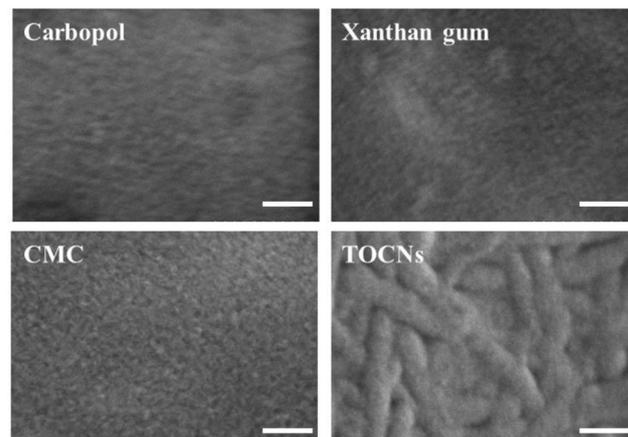
**Fig. 3** Nanometer-resolution structures of CNFs obtained in one-pot over Siliacat TEMPO and other water-soluble polymers obtained *via* high resolution imaging using FE-SEM. Scale bar = 100 nm. [Reproduced from ref. 14, Creative Commons Attribution (CC BY) license].
