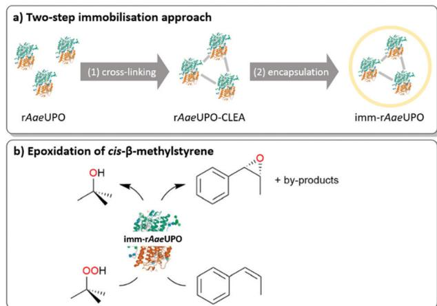
**Scheme 2** (a) Overview of the utilised immobilisation approach consisting of CLEA formation and alginate confinement. (b) Epoxidation of *cis*- $\beta$ -methylstyrene by immobilised *rAaeUPO* with *tert*-butyl hydroperoxide (*t*BuOOH) as oxidant.
