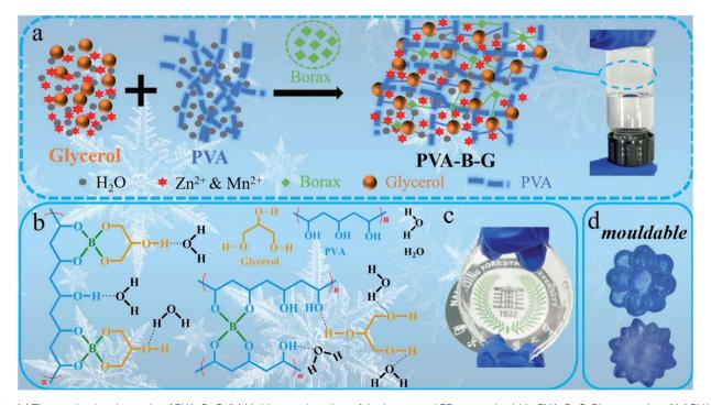
Fig. 1 (a) The synthesis schematic of PVA-B-G. (b) Multi-complexation of the integrated 3D network within PVA-B-G. Photographs of (c) PVA-B-G film and (d) PVA-B-G moulded into desirable shapes.
