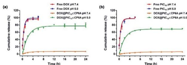
Fig. 3 Time dependent release of (a) DOX and (b) PtC<sub>10</sub> from DOX@PtC<sub>10</sub><CP6A in PBS at different pH (mean  $\pm$  SD,  $n = 3$ ). Concentrations at any given time point were determined by HPLC. See the ESI for details.†
