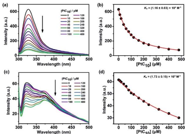
Fig. 1 Fluorescence spectra of CP6A ( $1.0 \times 10^{-5}$  M) in aqueous PBS (a) pH 7.4 and (c) pH 5.0 recorded in the presence of different concentrations of PtC<sub>10</sub> at 298 K. (b) and (d) nonlinear least-squares analyses used to calculate the  $K_a$  value.
