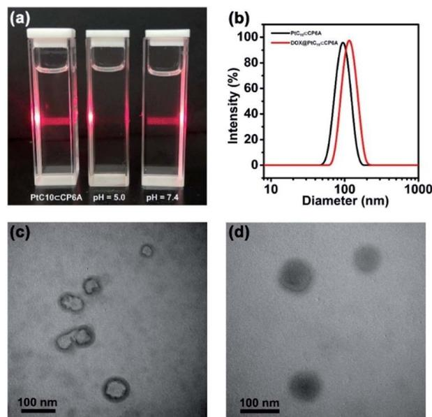
Fig. 2 (a) Tyndall effect seen for PtC<sub>10</sub>⊂CP6A aggregates prepared in aqueous solutions of different pH. (b) DLS data for PtC<sub>10</sub>⊂CP6A and DOX@PtC<sub>10</sub>⊂CP6A (298 K, scattering angle = 90°). TEM images: vesicles self-assembled from (c) PtC<sub>10</sub>⊂CP6A and (d) DOX@PtC<sub>10</sub>⊂CP6A ([CP6A] = 0.05 mM and [PtC<sub>10</sub>] = 0.10 mM).
