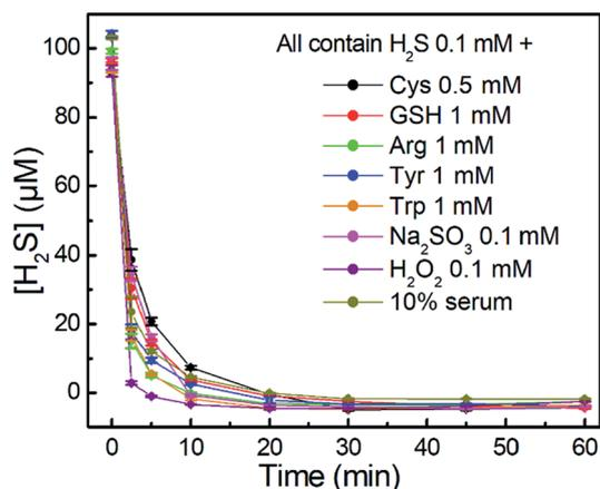
Fig. 6 Time-dependent H<sub>2</sub>S-scavenging curves of **NBD-S8** (110 μM) in the presence of other species (inset) and H<sub>2</sub>S (100 μM). The H<sub>2</sub>S concentrations were measured using MBA. The results are expressed as mean ± S.D. (*n* = 3).
