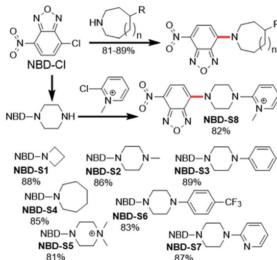
Fig. 2 Synthesis of NBD amines **NBD-S1** to **NBD-S8**. The C–N bond cleaved by H<sub>2</sub>S-mediated thiolysis is highlighted in red in each structure.
