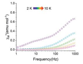
Fig. 11 Temperature dependence of the out-of-phase component of the molar ac magnetic susceptibility ( $\chi_{\rm M}^{\prime\prime}$ ) of 2-py (H=0 T, T=2-10 K).
