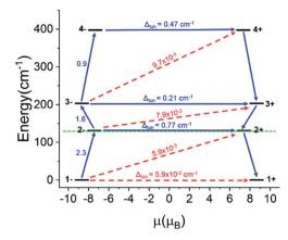
Fig. 14 Calculated barrier for magnetization reversal for Ho(2). The doublet states are arranged according to the values of their magnetic moments. The numbers at each arrow show the corresponding matrix element of the transversal magnetic moment, whereas  $\Delta_{\text{tun}}$  is the intrinsic tunneling gap of the corresponding doublet.
