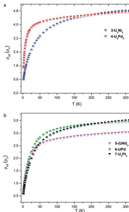
Fig. 6 Variable-temperature effective magnetic moment data. (a) Magnetic moment per molecule for **3-U<sub>2</sub>Ni<sub>2</sub>** and **4-U<sub>2</sub>Pd<sub>2</sub>**. (b) Magnetic moment per uranium ion for **5-(UNi)<sub>n</sub>**, **6-UPd**, and **7-U<sub>2</sub>Pt<sub>3</sub>**.
