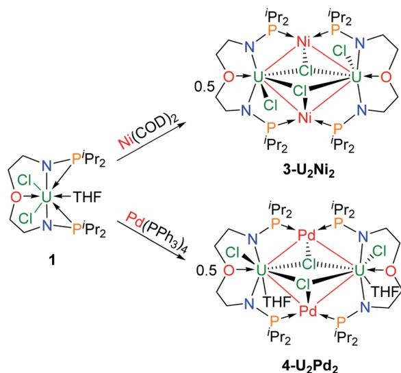
Scheme 2 Synthesis of heterometallic clusters with multiple U–Ni (**3-U<sub>2</sub>Ni<sub>2</sub>**) and U–Pd (**4-U<sub>2</sub>Pd<sub>2</sub>**) bonds.
