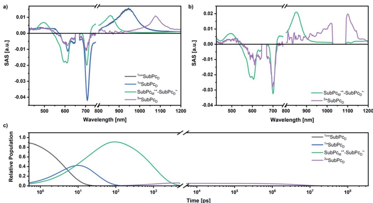
Fig. 10 SAS obtained by global target analysis of *syn*-SubPc 1 in PhCl after 656 nm laser excitation of (a) femtosecond and (b) nanosecond transient absorption data. (c) Calculated population profiles (the break marks the crossing from the femtosecond to the nanosecond setup).
