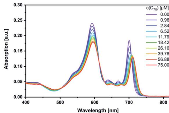
Fig. 5 Steady-state absorption spectra of *syn*-SubPc 1 ( $1.5 \times 10^{-6}$  M) in toluene with increasing amount of C<sub>70</sub> (0–75 μM).
