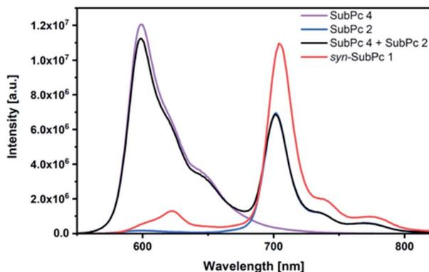
Fig. 4 Steady-state fluorescence spectra of *syn*-SubPc 1 ( $1.5 \times 10^{-6}$  M), dimer-SubPc 2 ( $1.5 \times 10^{-6}$  M) and monomer-SubPc 4 ( $3.0 \times 10^{-6}$  M) in toluene. The black spectrum relates to that of a 1 : 2 mixture of 2 and 4.  $\lambda_{\text{ex}} = 530$  nm.
