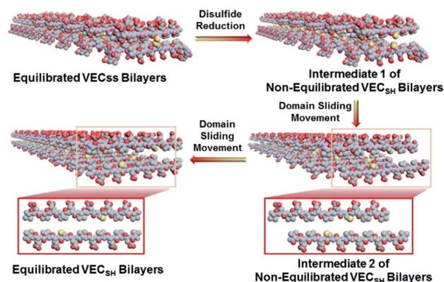
Fig. 5 Schematic representation of the mechanically dynamic process within the mechanically dynamic hydrogel  $\text{VEC}_{\text{SH}}\text{-MD}$  upon reduction of disulfide bonds and the resulting directional sliding movement promoted by the thermodynamically favourable hydrophobic collapse transition. The included molecular graphics are produced only for illustration.
