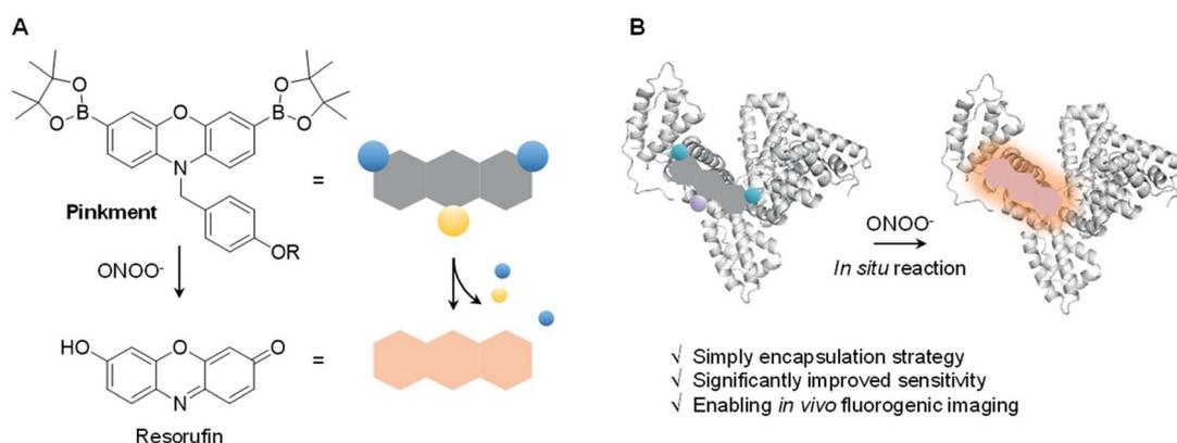
**Scheme 1** (A) Reaction mechanism of **Pinkment-OAc** (R = Ac) and **Pinkment-OH** (R = H) in the presence of  $\text{ONOO}^-$ . (B) Human serum albumin (HSA)-encapsulation of **Pinkment** enabling the detection of  $\text{ONOO}^-$  *in vitro* and *in vivo*.
