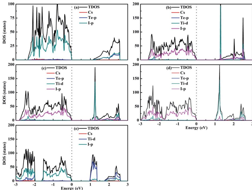
Fig. 7 Density of states of (a)  $\text{Cs}_2\text{TeI}_6$ , (b)  $\text{Cs}_2\text{Te}_{0.75}\text{Ti}_{0.25}\text{I}_6$ , (c)  $\text{Cs}_2\text{Te}_{0.50}\text{Ti}_{0.50}\text{I}_6$ , (d)  $\text{Cs}_2\text{Te}_{0.25}\text{Ti}_{0.75}\text{I}_6$ , and (e)  $\text{Cs}_2\text{TiI}_6$ .
