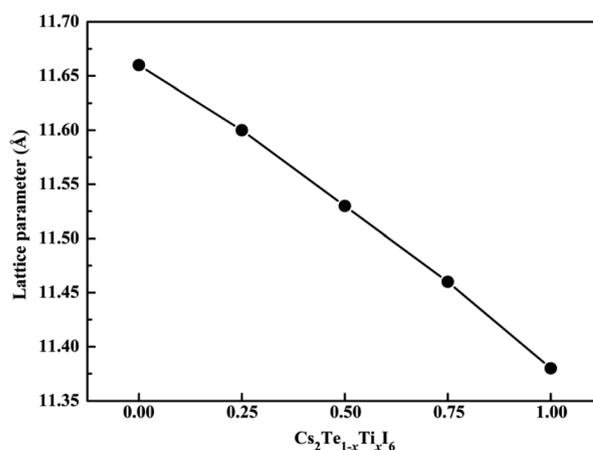
Fig. 2 The lattice constants of the  $\text{Cs}_2\text{Te}_{1-x}\text{Ti}_x\text{I}_6$  solid solutions.
