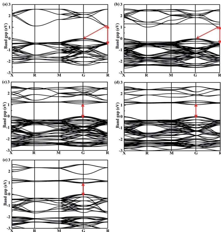
**Fig. 5** Calculated band structures of double perovskites along the  $X-R-M-G-R$  path for (a)  $\text{Cs}_2\text{TeI}_6$ , (b)  $\text{Cs}_2\text{Te}_{0.75}\text{Ti}_{0.25}\text{I}_6$ , (c)  $\text{Cs}_2\text{Te}_{0.50}\text{Ti}_{0.50}\text{I}_6$ , (d)  $\text{Cs}_2\text{Te}_{0.25}\text{Ti}_{0.75}\text{I}_6$ , and (e)  $\text{Cs}_2\text{TiI}_6$ .
