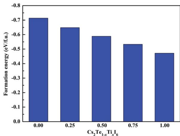
Fig. 3 Calculated formation energies of the Cs<sub>2</sub>Te<sub>1-x</sub>Ti<sub>x</sub>I<sub>6</sub> solid solutions.
