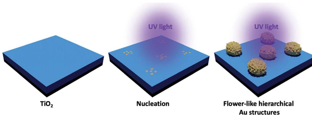
Fig. 1 Schematic representation of the photocatalytic deposition of Au structures on the TiO<sub>2</sub> thin film surface.
