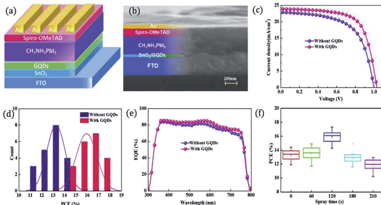
Fig. 19 (a) schematic diagram of perovskite solar cell. (b) Cross sectional SEM image of perovskite structure. (c)  $J$ - $V$  curves of the PSC based on  $\text{SnO}_2$  with and without GQDs. (d) Statistic histogram of the power conversion efficiency (PCE) (e) external quantum efficiency spectra. (f) PCE tendency with different time period. Reproduced with permission from ref. 211, copyright 2019, Elsevier.
