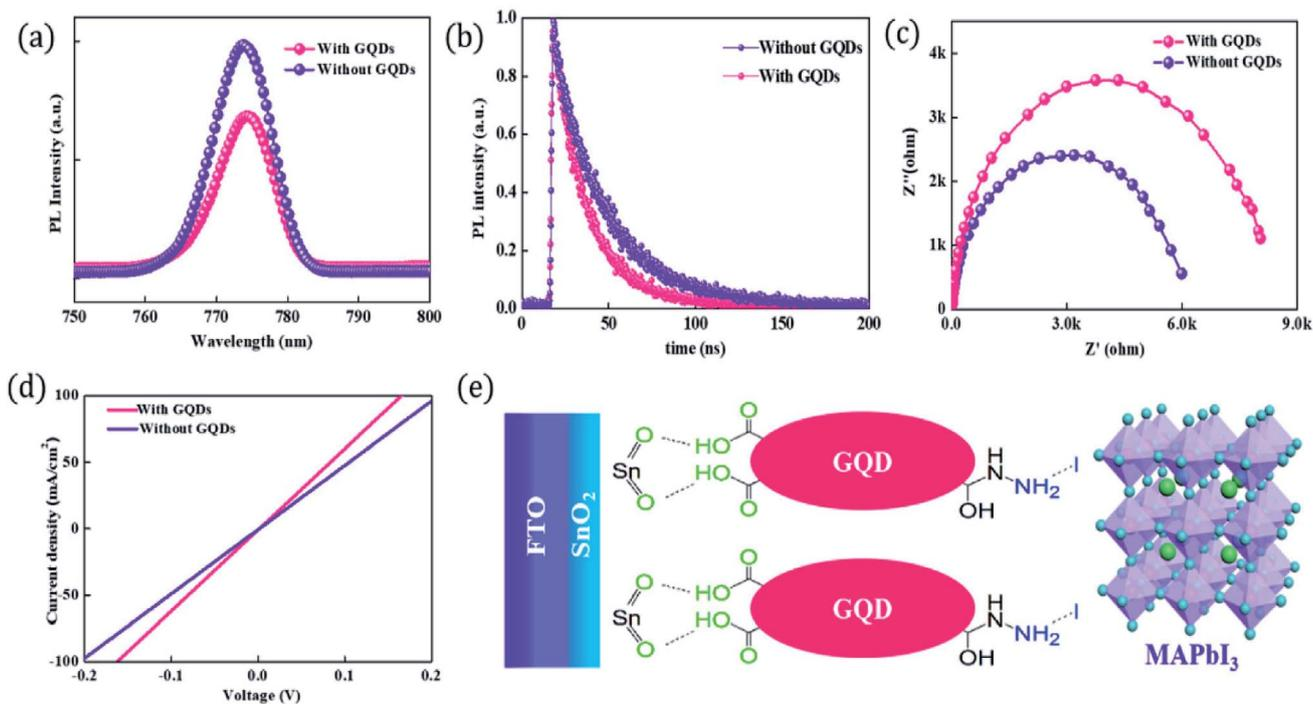
Fig. 20 (a and b) Steady-state PL and TRPL spectrum of perovskite structure. (c) Electrochemical impedance spectrum of perovskite structure (d)  $J$ - $V$  curves of the device under light environment. (e) Schematic diagram of the interfacial reaction between  $\text{SnO}_2/\text{GQDs}$  and  $\text{GQDs}/\text{perovskite}$ . Reproduced with permission from ref. 211, copyright 2019, Elsevier.
