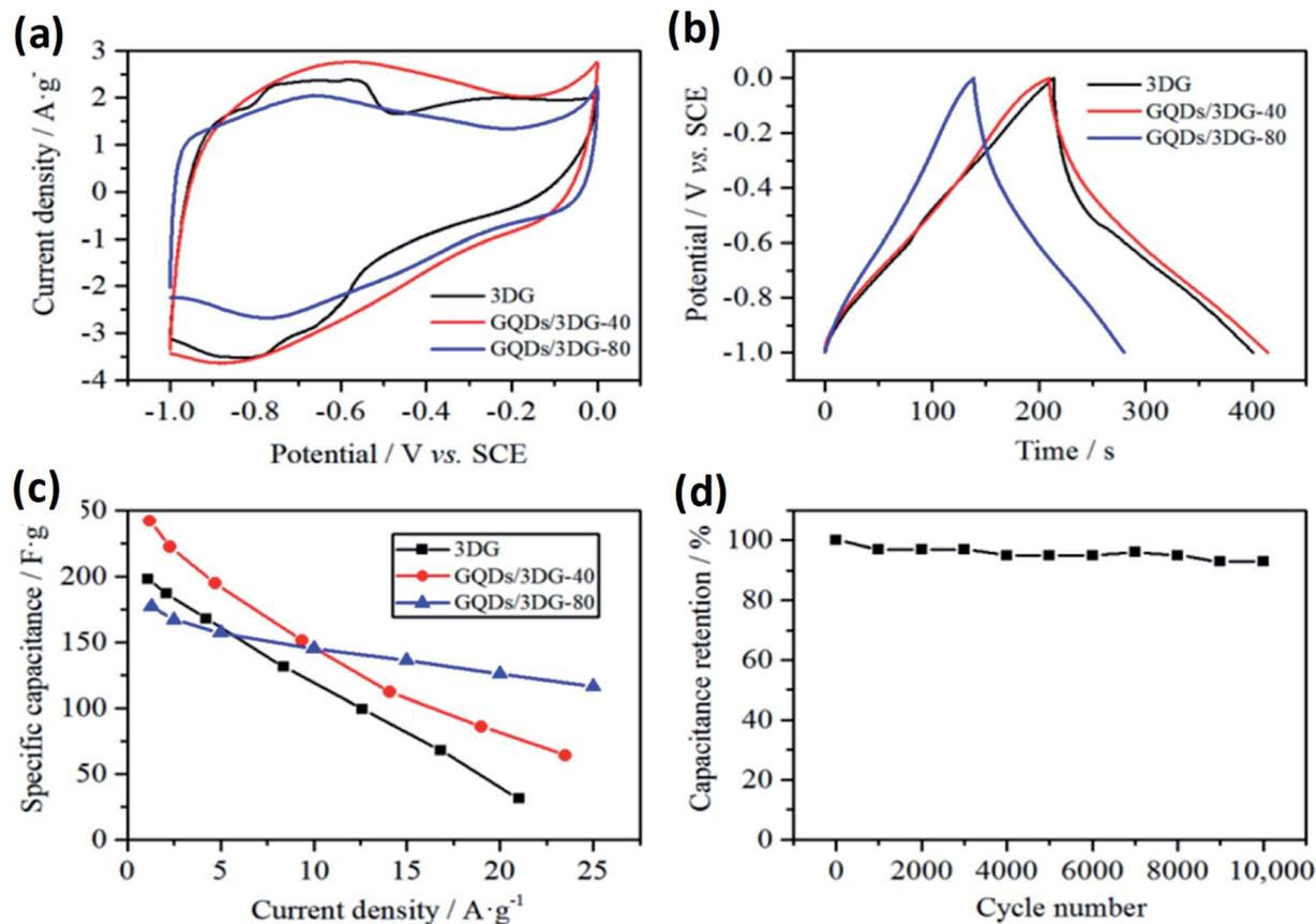
Fig. 18 (a) Cyclic voltammety curve at a scan rate of  $10 \text{ mV s}^{-1}$  (b) charge/discharge curves at different current densities with different compositions, respectively (c) specific capacitance versus current densities and (d) cycling stability at a current density of  $24 \text{ A g}^{-1}$  for the composite material. Adapted from ref. 183, copyright 2019, MDPI publications.
