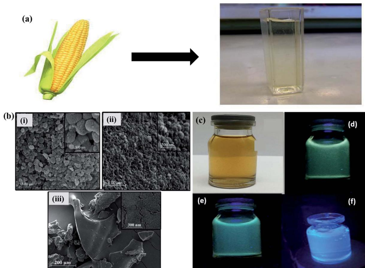
Fig. 8 (a) Schematic diagram of GQDs synthesis through green chemistry (b) SEM images of as-prepared GQDs,  $\text{TiO}_2$  and GQDs/ $\text{TiO}_2$  composite, (c) as-synthesized GQDs under normal light and (d–f) UV light. Reproduced with permission from ref. 85, copyright 2017, Elsevier.
