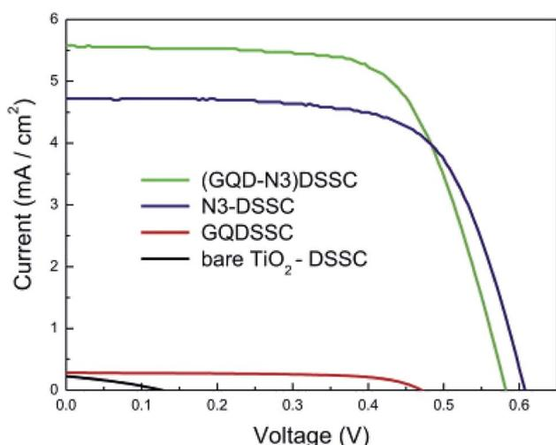
Fig. 22  $J$ - $V$  characteristics curves of DSSCs with bare GQD,  $N_3$ ,  $TiO_2$  and combination of GQD and  $N_3$  were taken under 1 sun illumination intensity. Reproduced with permission from ref. 214, copyright 2015, Elsevier.
