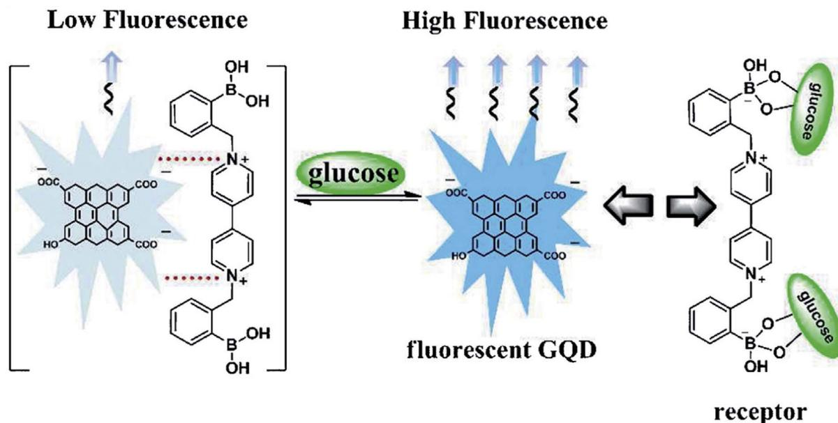
Fig. 10 Sensing mechanism based on BBV receptor and fluorescent GQDs. Reproduced with permission from ref. 116, copyright 2013, The Royal Society of Chemistry.
