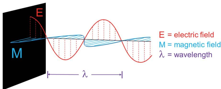
Fig. 1 General schematic for microwave energy.
