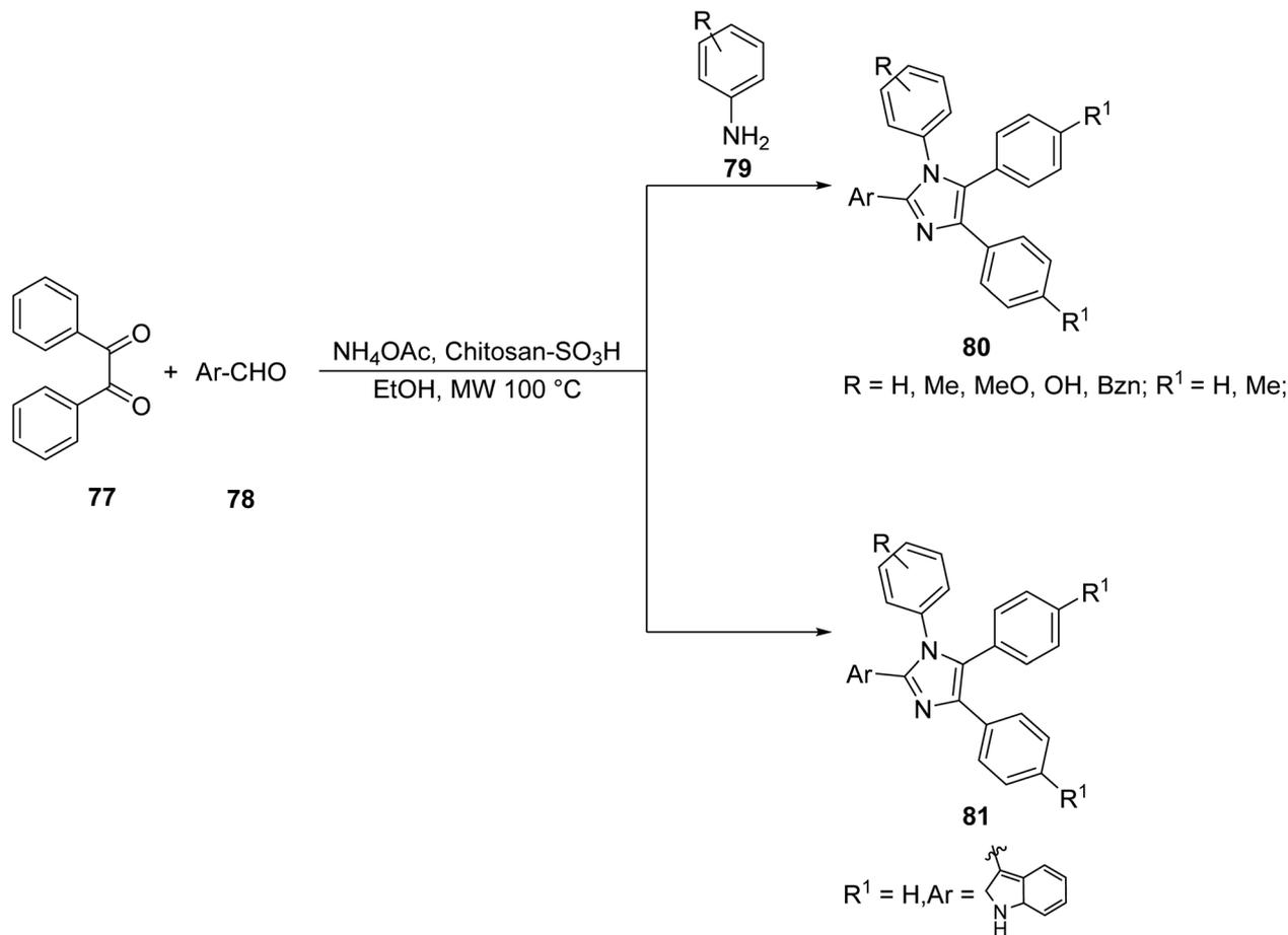
Scheme 5 Synthesis of polycyclic imidazole derivatives via benzyl.<sup>64</sup>Table 6 Comparison of conventional versus microwave methods in the synthesis of substituted imidazoles. Microwave irradiation was conducted at 5–10 W and 100 °C<sup>64</sup>
