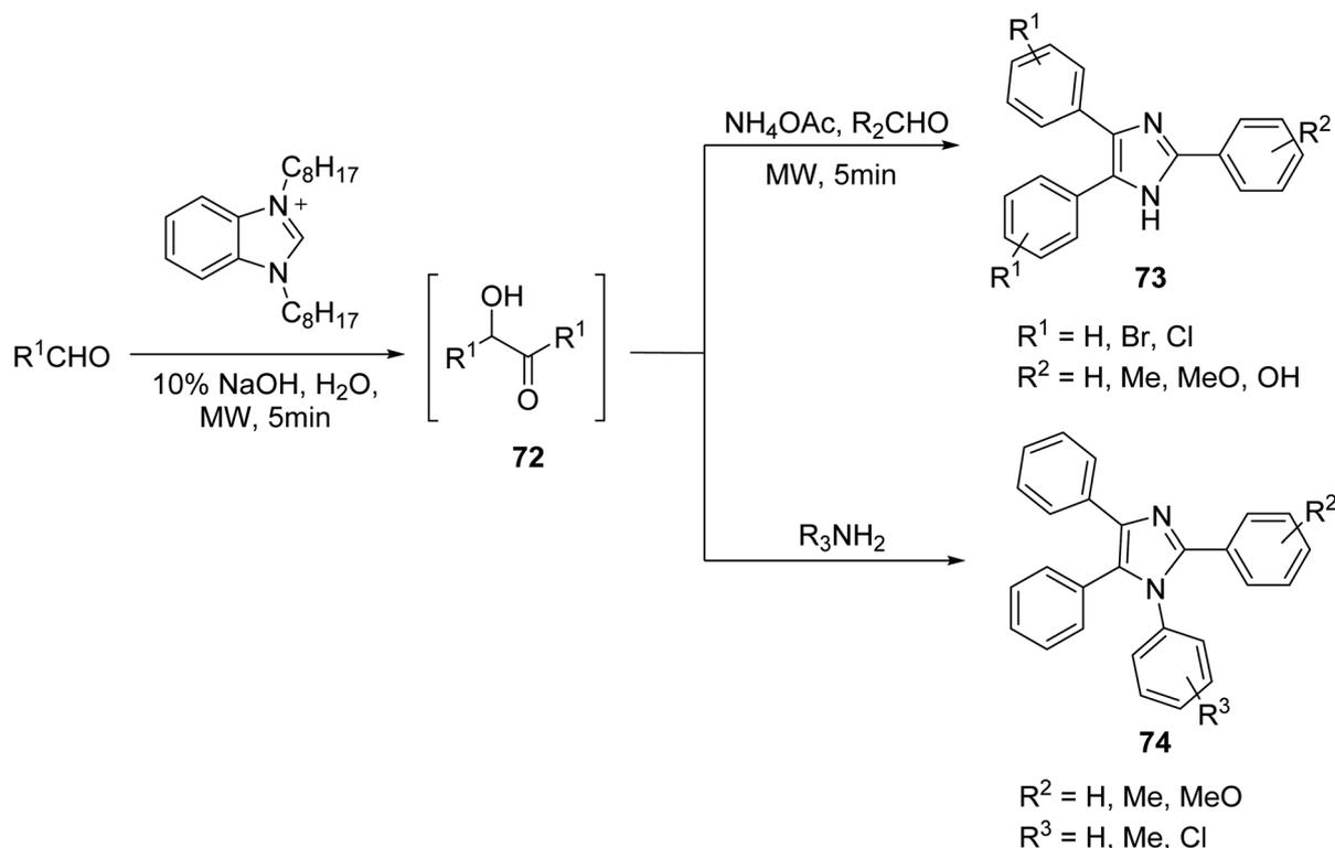
**Scheme 4** Synthesis of tri- and tetra-substituted imidazole analogs via arylaldehydes.<sup>62</sup>
