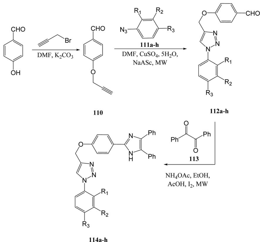
Scheme 9 Synthesis of imidazole containing 1,2,3-triazole derivatives via 4-hydroxy benzaldehyde.<sup>100</sup>
