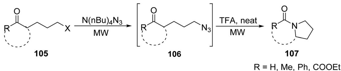
Scheme 8 Synthesis of fused cyclic lactam derivatives *via* keto chloride.<sup>92</sup>
