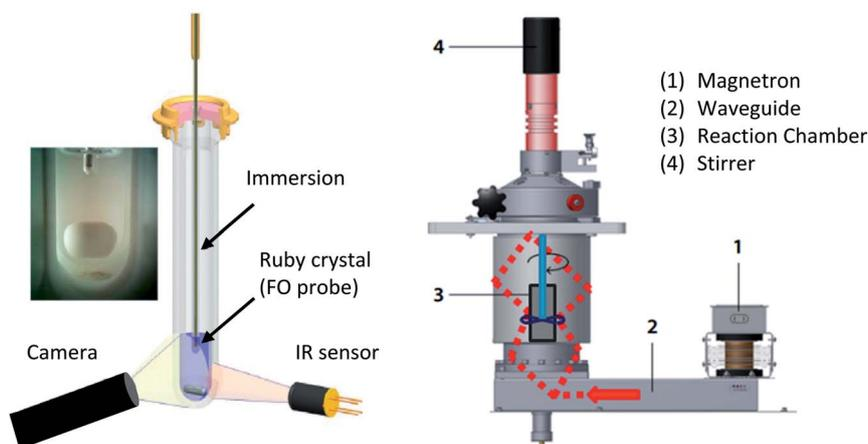
Fig. 2 (Left): scheme of a monomode reactor.<sup>17</sup> (Right): scheme of a multi-mode reactor.<sup>16</sup>
