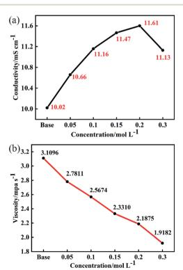
Fig. 1 Effect of different concentrations of LiDFP on conductivity (a) and viscosity (b) of electrolyte.
