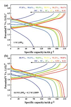
Fig. 4 The rate performance of NCM811/Li cells with (a) the blank electrolyte containing 1 M LiPF $_6$ ; and (b) the dual-salt electrolyte containing 0.8 M LiPF $_6$  + 0.2 M LiDFP.
