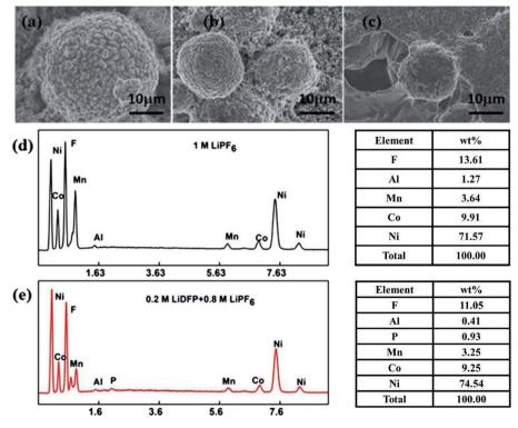
Fig. 8 SEM images of the NCM 811 electrode: fresh (a) and after 130 cycles in (b) the dual-salt electrolyte containing  $0.8 \text{ M LiPF}_6 + 0.2 \text{ M LiDFP}$ , (c) the blank electrolyte containing  $1 \text{ M LiPF}_6$ . The corresponding EDS analysis of surface element distribution of the NCM 811 electrode after 130 cycles in blank electrolyte (d) and dual-salt electrolyte (e).
