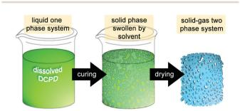
Fig. 7 Schematic preparation of aerogels.
