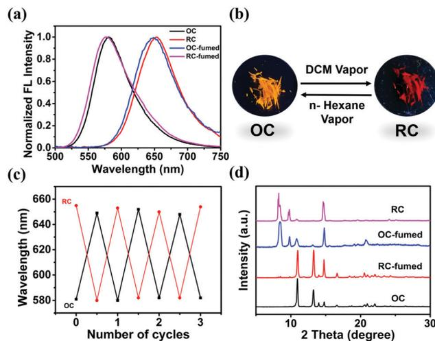
Fig. 4 (a) Normalized FL spectra ( $\lambda_{ex} = 400$  nm) of the original **OC** and **RC** and the corresponding fumed samples, **OC-fumed** and **RC-fumed**, under excitation at 365 nm. (b) FL images of the crystals before and after vapor fuming. (c) Cyclic FL emission of the crystal-to-crystal switch. (d) Powder diffraction pattern of the original and fumed crystals.
