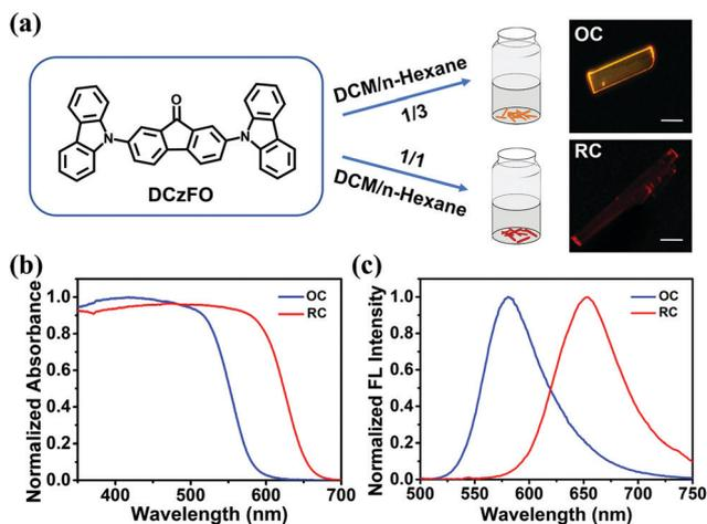
Fig. 2 (a) Schematic illustration of the preparation process of the polymorphs and the FL micrographs of **OC** and **RC** crystals irradiated under a UV lamp (365 nm). (b) Normalized UV-vis and (c) FL spectra ( $\lambda_{\text{ex}} = 400 \text{ nm}$ ) of **OC** (blue line) and **RC** (red line). Scale bar: 200  $\mu\text{m}$ .
