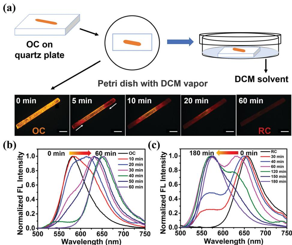
Fig. 5 (a) Schematic vapor fuming process of **OC** in a Petri dish with DCM vapor and micrographs showing the crystal-to-crystal switching process upon vapor fuming under UV irradiation (365 nm). (b) Normalized FL spectra ( $\lambda_{\text{ex}} = 400$  nm) of **OC** at 10 minute intervals from 0 to 60 min. (c) Normalized FL spectra ( $\lambda_{\text{ex}} = 400$  nm) of **RC** at 10 minute fuming time intervals from 0 to 180 min. Scale bar: 200  $\mu\text{m}$ .
