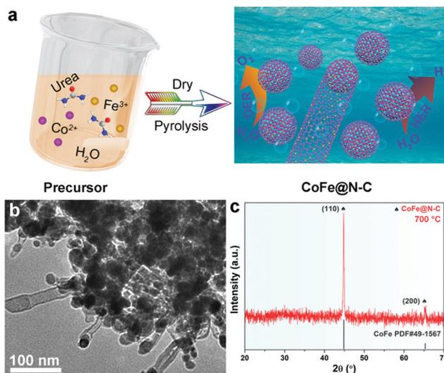
Fig. 1 (a) Schematic illustration of the synthetic procedure of the CoFe@N-C catalysts. (b) TEM image and (c) XRD pattern of the as-synthesized CoFe@N-C.
