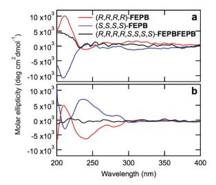
Fig. 3 Circular dichroism spectra of (R,R,R,R)-FEPB (red), (S,S,S,S)-FEPB (blue) and (R,R,R,R,S,S,S,S)-FEPBFEPB (black) in CH<sub>3</sub>CN. Concentrations are (a) 30  $\mu M$  and 15  $\mu M$  for the tetramers and octamer, respectively; (b) 150 µM and 75 µM for the tetramers and octamer, respectively. The spectra were smoothed (Savitzky-Golay, 13-point, second order polynomial).
