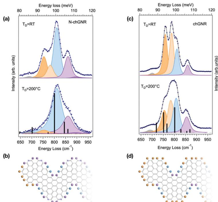
**Fig. 3** Comparison between the HREEL spectra of N-doped (a) and pristine (c) chevron-type GNRs, obtained by deposition at  $T_D = 200$  °C and at RT. The corresponding fitting components are shown as shaded curves, while calculated modes are displayed as black bars. The corresponding molecular schemes, showing the structure of the termini, are reported in (b) and (d), respectively. The top spectrum in (a) is also reported in the right panel of Fig. 1.
