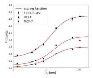
Fig. 2 The logarithm of effective viscosity experienced by nanoprobes of radii  $r_p$  moving in the ECM of HeLa, MCF-7, and fibroblast spheroids. Error bars correspond to the standard deviations (N > 30). The fit of a length-scale dependent viscosity model (eqn (2)) is presented as a solid line. The fitting parameters are listed in Table 2. The diffusion coefficient of any inert probe within the ECM of studied cell line spheroids can be estimated from the presented length-scale dependent model.
