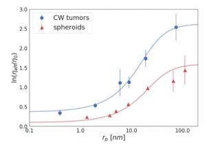
Fig. 7 The logarithm of the effective viscosity experienced by the nanoprobes of radii  $r_{\rm p}$  moving in the CW tumours<sup>32</sup> and spheroids (the average value for all 3 cell lines). The solid lines calculated from eqn (2). The error bars correspond to the maximal error calculated on the basis of standard deviations of measurements.
