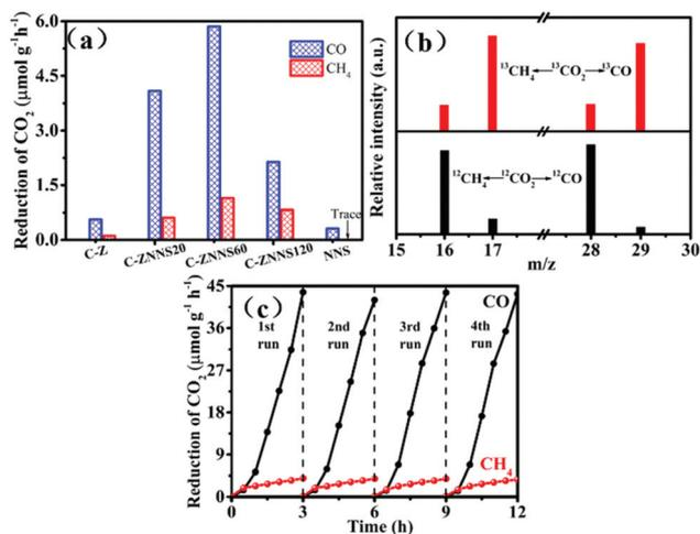
Fig. 6 (a) Photocatalytic  $\text{CO}_2$  reduction performances of all samples. (b) CO and  $\text{CH}_4$  mass spectra of C-ZNNS60. (c) Cyclic  $\text{CO}_2$  reduction curves for CO and  $\text{CH}_4$  yield (350 W,  $\text{NaHCO}_3 = 1$  mmol).
