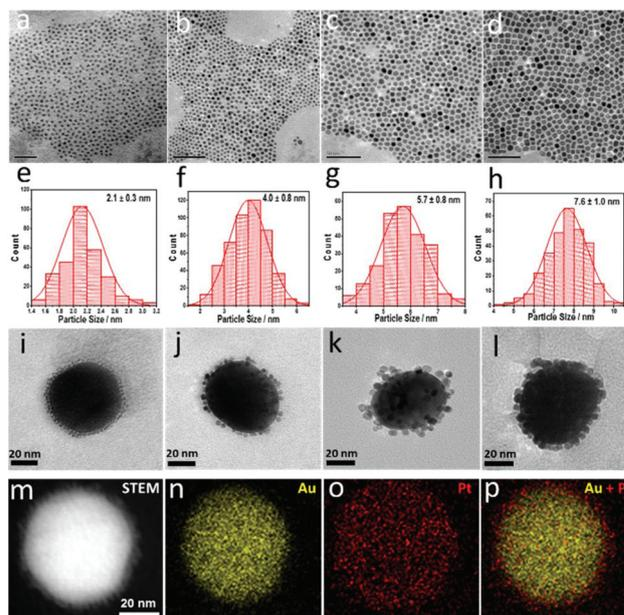
**Fig. 1** (a)–(d) TEM images of Pt nanoparticles with different sizes. Their size distributions are shown in (e)–(h), respectively. (i)–(l) TEM images of the Pt-on-Au satellite nanostructure catalysts. 55 nm Au NPs (larger particles) are surrounded by Pt NPs (smaller ones) shown in (a)–(d) *via* electrostatic self-assembly. (m)–(p) High-angle annular dark field scanning transmission electron microscopy (HAADF-STEM) image and elemental maps of Pt (2.1 nm)-on-Au.
