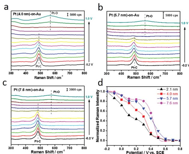
Fig. 4 (a)–(c) are the electrochemical SERS spectra for CO electrooxidation in 0.1 M HClO<sub>4</sub> on Pt-on-Au with a Pt particle size of 4.0 nm, 5.7 nm, and 7.6 nm, respectively. (d) Normalized Raman intensity of Pt–CO bands as a function of the potential.
