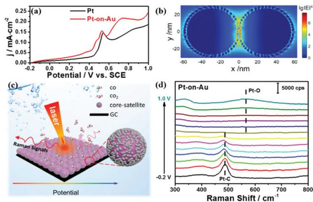
**Fig. 2** (a) CO stripping voltammograms for Pt and Pt-on-Au core-satellite nanocatalysts in 0.1 M HClO<sub>4</sub> at a scan rate of 20 mV s<sup>-1</sup>. (b) 3D-FDTD simulation for a pair of Pt-on-Au nanocomposites. (c) A schematic diagram of the *in situ* electrochemical SERS study of CO electrooxidation. (d) The electrochemical SERS spectra for CO electrooxidation in 0.1 M HClO<sub>4</sub> on Pt (2.1 nm)-on-Au core-satellite nanocatalysts.
