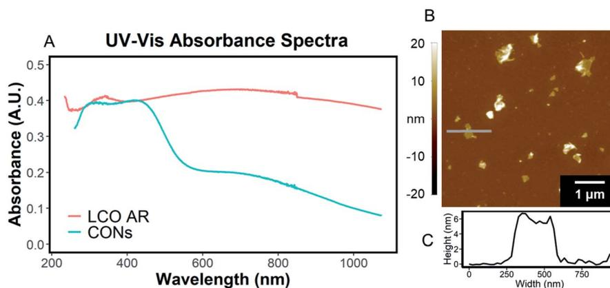
**Fig. 4** (A) UV-Vis absorbance spectra of a solution of CONs (blue) and lithium cobalt oxide powder (orange). CONs (prepared from 1 day 3 M HCl and 1 day 0.044 M TMAOH treatment) were suspended in 0.044 M TMAOH and were separated from bulk powder *via* centrifugation. Lithium cobalt oxide was suspended in polyethylene glycol to prevent sedimentation. (B) AFM image and (C) line scan height profile of the same solution of CONs drop cast onto a clean mica substrate.
