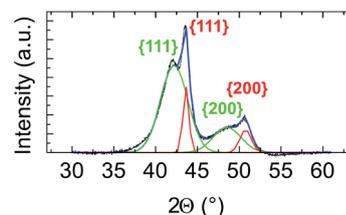
Fig. 2  $\text{Ni}_3\text{Pt}$  (75 : 25) elaborated at 225 °C core-shell PXRD patterns, deconvolution of the different peaks (in blue) and indexing of peaks assuming that the core is the NiPt solid solution in green and the shell, the  $\text{Ni}_3\text{Pt}$  solid solution in red.
