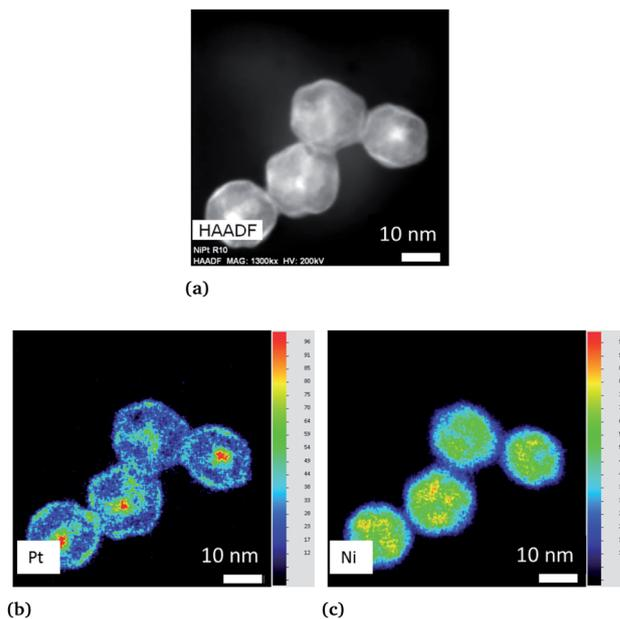
Fig. 1  $\text{Ni}_3\text{Pt}$  colloidal synthesis performed at 225 °C. (a) STEM-HAADF image and chemical mappings using EDX mode with the concentration scale demonstrate that (b) Pt ( $L_z$  line) is predominantly located in the core and (c) Ni ( $K_z$  line) mainly in the shell.
