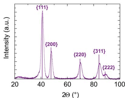
Fig. 7 Sample B PXRD pattern analysed assuming an FCC structure with the lattice parameter equal to  $(0.380 \pm 0.003)$  nm. The crystalline domain size is measured from the peak width to be equal to  $(4.5 \pm 0.5)$  nm. The diffraction peak indexing related to the theoretical NiPt FCC structure.
