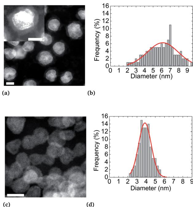
Fig. 4 STEM-HAADF micrographies and size distribution histograms of  $\text{Ni}_3\text{Pt}$  NPs elaborated at (a and b)  $200 \text{ }^\circ\text{C}$  showing a core–shell structure and an observable organic layer surrounding the particle in the magnified image in the inset and at (c and d)  $280 \text{ }^\circ\text{C}$  showing alloyed particles (scale bar = 5 nm).
