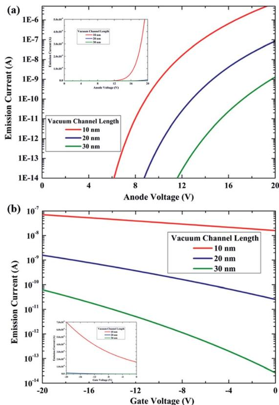
Fig. 3 The (a) output characteristic and (b) transfer characteristic curves of nanoscale vacuum channels with various lengths in the logarithmic form. The insets show the  $I$ - $V$  curves in the linear form.
