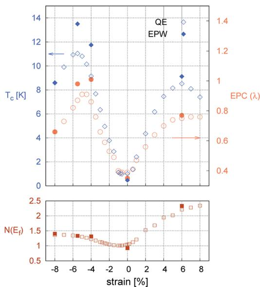
Fig. 3 Change in transition temperature  $T_c$  [K], EPC constant ( $\lambda$ ), and DOS at the Fermi level ( $N(E_F)$ ) [states/spin/eV/unit cell] as a function of strain. Opened and closed dots refer to converged values in coarse  $k$ - and  $q$ -meshes from Quantum Espresso and in dense  $k$ - and  $q$ -meshes from EPW, respectively. Both results indicated well-converged conditions.
