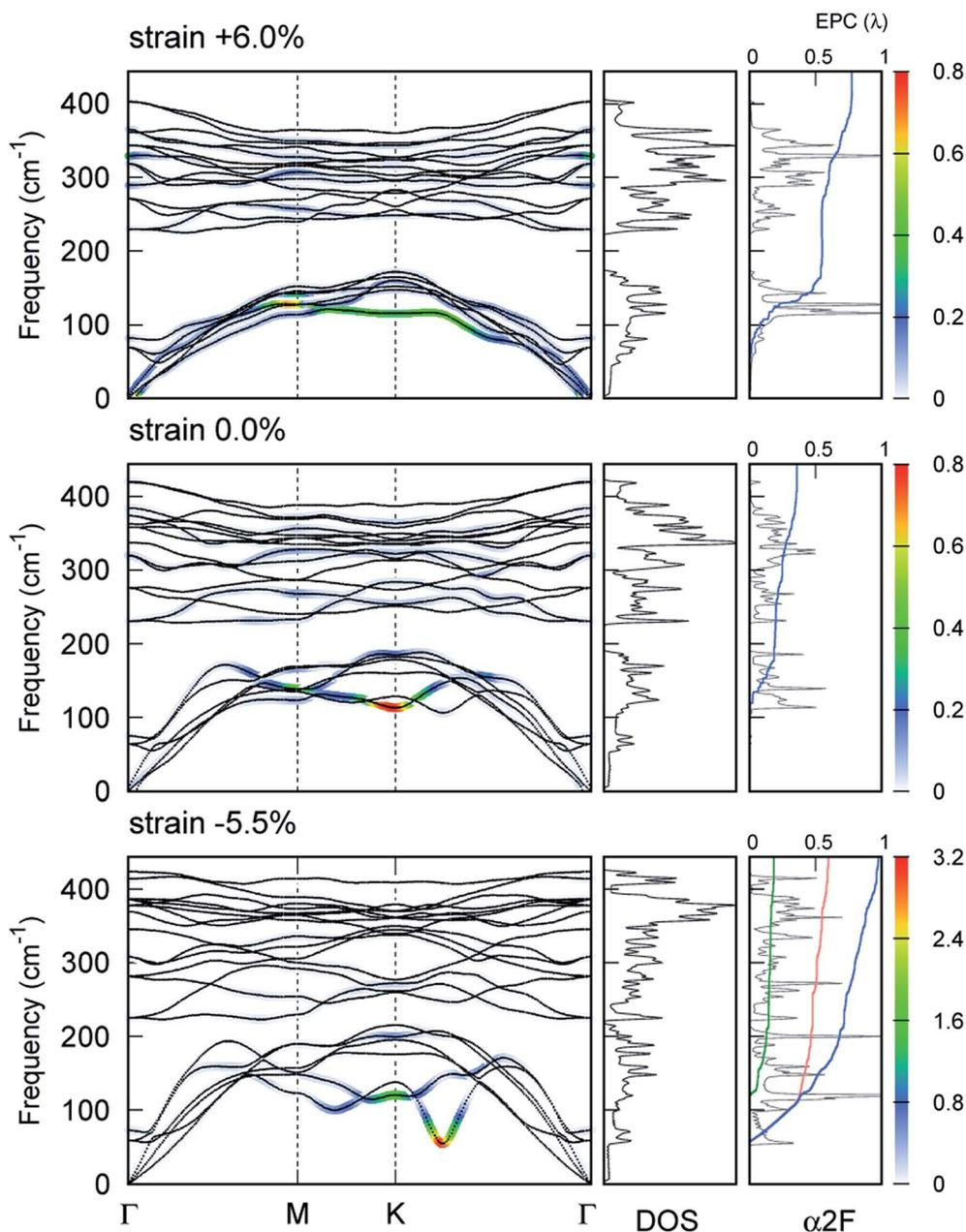
Fig. 5 Phonon dispersion at zero strain (middle) and at the highest  $T_c$  with tensile (top) and compressive (bottom) strains together with phonon density of states (DOS) and Eliashberg spectral function ( $\alpha^2F$ ). The color corresponds to the strength of the EPC constant. Integrated EPC as a function of frequency is shown (blue) together with an interband component (orange) and a pocket-involved intraband component (green) resolved through EPC.
