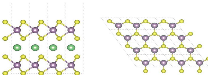
Fig. 1 Side view (left) and top view (right) of the Li-intercalated bilayer MoS<sub>2</sub> structure. Purple, yellow, and green spheres denote Mo, S, and Li, respectively.
