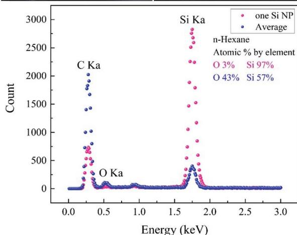
Fig. 7 The femtosecond laser-synthesized Si nanoparticles in *n*-hexane. ( $N = 1000$ ,  $F = 10.46 \text{ J cm}^{-2}$ ). The TEM bright-field image, SAED pattern (upper right) and dark-field images related to different diffracted electron beams along the 1<sup>st</sup> and 2<sup>nd</sup> ring. The EDX spectrum from several small Si NPs and one Si NP.
