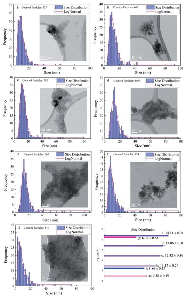
Fig. 3 Ferret size distribution study of femtosecond laser synthesized silicon nanoparticles ( $N = 1000$ , 1 kHz): (a) ethanol,  $F = 2.94 \text{ J cm}^{-2}$ , (b) ethanol,  $F = 4.90 \text{ J cm}^{-2}$ , (c) ethanol,  $F = 6.86 \text{ J cm}^{-2}$ , (d) ethanol,  $F = 8.82 \text{ J cm}^{-2}$ , (e) ethanol,  $F = 10.78 \text{ J cm}^{-2}$ , (f) 2-butanol,  $F = 4.42 \text{ J cm}^{-2}$ , and (g) *n*-hexane,  $F = 10.46 \text{ J cm}^{-2}$ .
