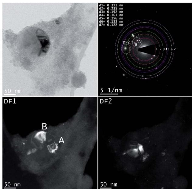
Fig. 5 The femtosecond laser-synthesized Si nanoparticles in ethanol. ( $N = 1000$ ,  $F = 10.78 \text{ J cm}^{-2}$ ). The BF-TEM image (upper left), SAED pattern (upper right) and the DF-TEM images related to different diffracted electron beams along the 1<sup>st</sup> and 3<sup>rd</sup> ring.
