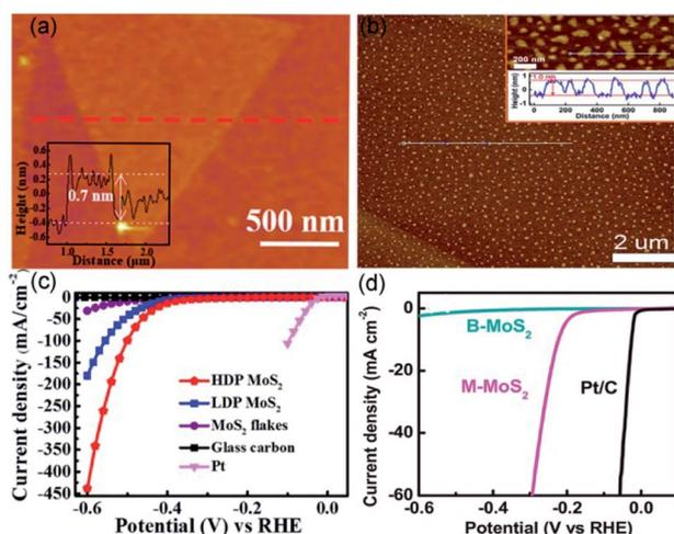
Fig. 3 AFM images and the corresponding heights of (a) HDP-MoS<sub>2</sub> precursor and (b) M-MoS<sub>2</sub>. The polarization curves of (c) HDP-MoS<sub>2</sub> and (d) M-MoS<sub>2</sub> in comparison with other catalysts. (a and c) Reproduced from ref. 47. Copyright 2018, American Chemical Society. (b and d) Reproduced from ref. 71. Copyright 2019, Elsevier.
