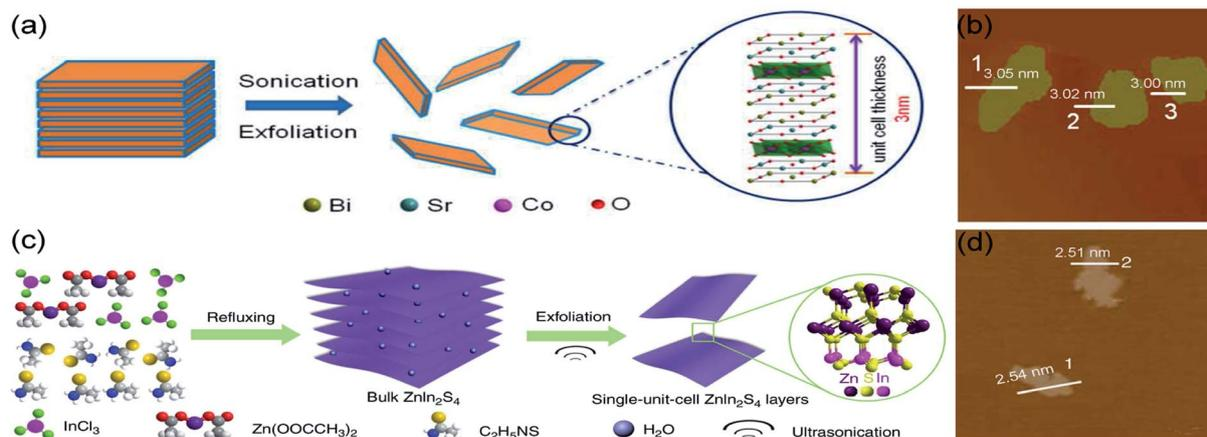
Fig. 2 Schematic illustration of ultrasonic exfoliation of bulk (a) BSCO and (c)  $\text{ZnIn}_2\text{S}_4$ ; AFM images of single-unit-cell (b) BSCO and (d)  $\text{ZnIn}_2\text{S}_4$ . (a and b) Reproduced from ref. 5. Copyright 2018, American Chemical Society. (c and d) Reproduced from ref. 61. Copyright 2017, Springer Nature.
