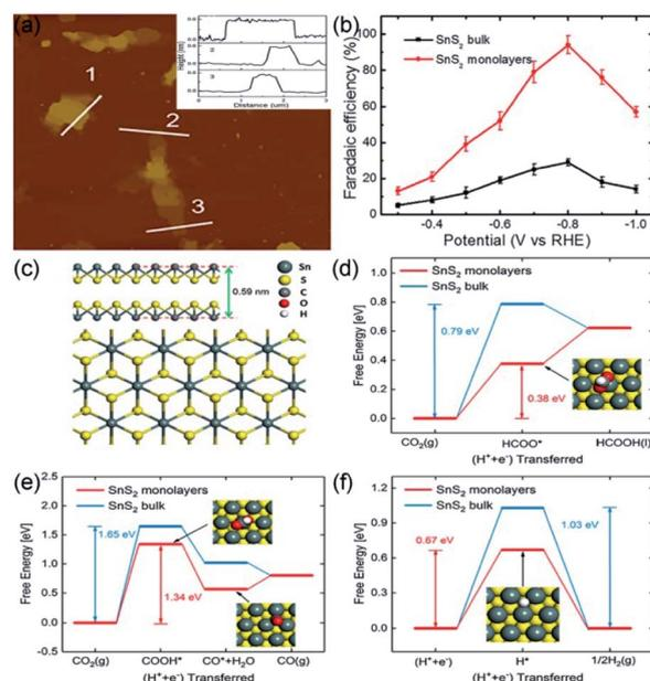
Fig. 6 (a) AFM image and the corresponding heights and (b) FEs of formate over SnS<sub>2</sub> monolayer at various applied potentials. (c) Atomic side and top models of single-unit-cell SnS<sub>2</sub>. (d and e) Free energy results of CO<sub>2</sub> reduction to (d) HCOOH and (e) CO by SnS<sub>2</sub> monolayer and bulk surface. (f) Free energy results of HER by SnS<sub>2</sub> monolayer and bulk surface. Reproduced from ref. 48. Copyright 2018, Elsevier.
