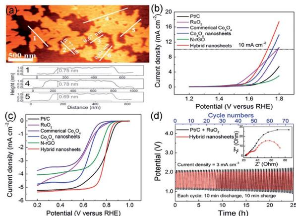
Fig. 8 (a) AFM image and the corresponding height profiles of Co<sub>3</sub>O<sub>4</sub>/N-rGO NS. (b) and (c) Linear sweep voltammetry curves of Co<sub>3</sub>O<sub>4</sub>/N-rGO, Co<sub>3</sub>O<sub>4</sub>-NS, N-rGO, commercial Co<sub>3</sub>O<sub>4</sub>, RuO<sub>2</sub>, and Pt/C. (d) Charge and discharge cycling curves of Co<sub>3</sub>O<sub>4</sub>/N-rGO and electrochemical impedance spectroscopy (EIS) spectrum of ZAB. Reproduced from ref. 84. Copyright 2018, Wiley-VCH.
