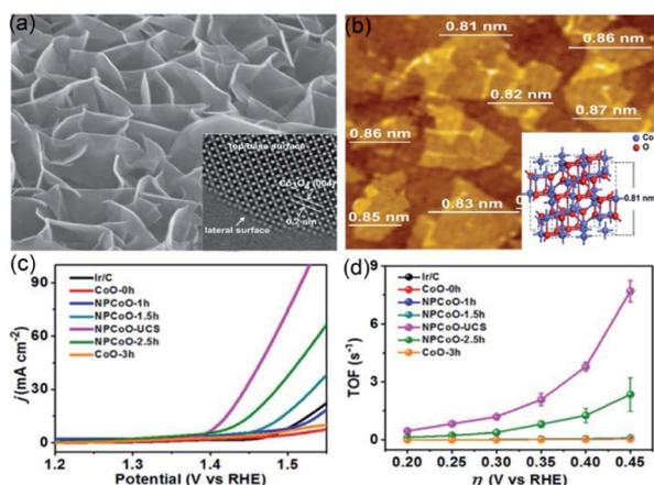
Fig. 5 (a) Low-magnification and high-resolution TEM images of NPCoO-UCSs. (b) Top-view AFM image of NPCoO-UCSs, the measurable thickness close to the inserting 3D model of standard Co<sub>3</sub>O<sub>4</sub> unit cell. (c) OER polarization curves of NPCoO-UCSs and other catalysts. (d) TOF vs. thickness curves of NPCoO-UCSs and other catalysts. Reproduced from ref. 44. Copyright 2018, Elsevier.
