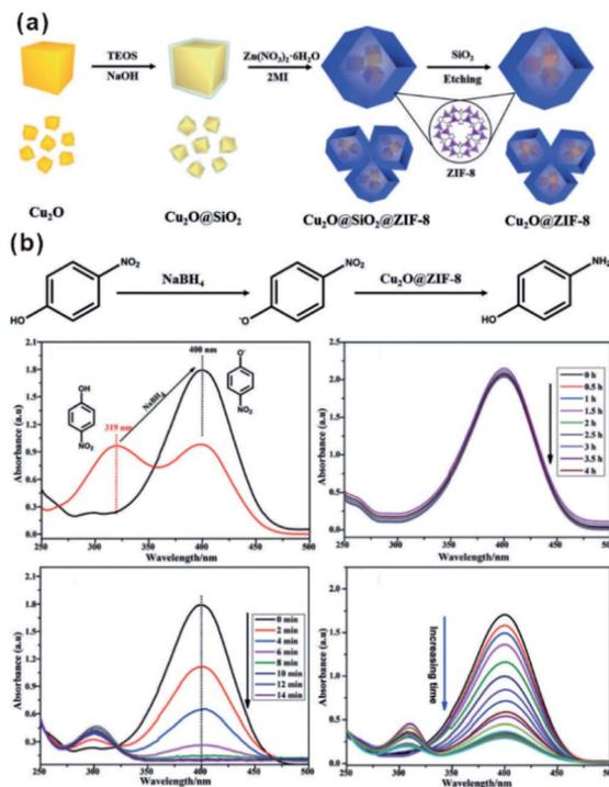
Fig. 8 (a) Schematic illustration of synthesis of the Cu<sub>2</sub>O@ZIF-8 composite, and (b) catalytic reduction equation of 4-nitrophenol to 4-aminophenol using Cu<sub>2</sub>O@ZIF-8. Reproduced with permission.<sup>86</sup> Copyright©2018 WILEY-VCH Verlag GmbH & Co. KGaA.
