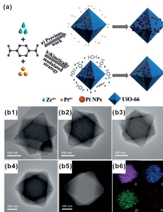
Fig. 7 (a) Incorporation of Pt NPs in MOFs through an *in situ* one-step strategy and a kinetically modulated *in situ* one-step strategy. (b1–b4) TEM images of Pt@UiO-66 nanocomposites prepared by different volume ratios of H<sub>2</sub>/air. A (b5 and b6) HAADF-STEM image and corresponding elemental mapping of Pt@UiO-66. Reproduced with permission.<sup>77</sup> Copyright©2016 WILEY-VCH Verlag GmbH & Co. KGaA.
