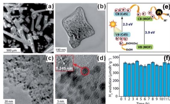
Fig. 23 (a) SEM images of CdS@ZAVCl and (b–d) TEM images of CdS@ZAVCl-MOF. (e) Mechanism of water splitting by the CdS@ZAVCl photocatalyst (30 mg) using 0.5 wt% co-catalyst Pt at  $\lambda > 420$  nm. (f) Stability tests of photocatalyst (CdS@ZAVCl-MOF) for 12 cycles of the water splitting reaction. Reproduced with permission.<sup>207</sup> Copyright©2014 American Chemistry Society.
