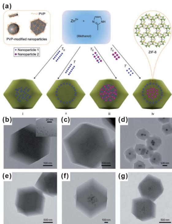
**Fig. 1** (a) Scheme of controlled encapsulation of NPs in ZIF-8 crystals. Transmission electron microscopy (TEM) images of hybrid crystals containing: (b) 3.4% 3.3 nm Pt NPs, (c) 0.7% 3.3 nm Pt NPs, (d) Ag cubes, (e) 13 nm Au NPs, (f) 13 nm Au and 34 nm Au NPs in the central area, and (g) subsequent 34 nm Au nanoparticle-rich cores and 13 nm Au nanoparticle-rich transition layers. Reproduced with permission.<sup>40</sup> Copyright©2012 Nature Publishing Group.
