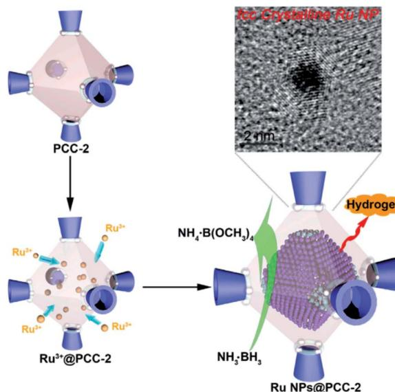
**Fig. 3** Scheme representing the synthesis of *fcc* Ru NPs via PCC-2 as the template. Reproduced with permission.<sup>57</sup> Copyright©2018 Elsevier Inc.
