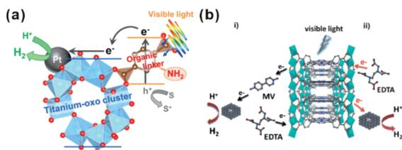
Fig. 22 Scheme illustrating the photocatalytic H<sub>2</sub> production reaction over (a) Pt/Ti-MOF-NH<sub>2</sub> and (b) Al-PMOF based on LCCT or LMCT mechanisms. Reproduced with permission.<sup>203</sup> Copyright©2012, 2015 American Chemistry Society. Reproduced with permission.<sup>204</sup> Copyright©2012 WILEY-VCH Verlag GmbH & Co. KGaA.
