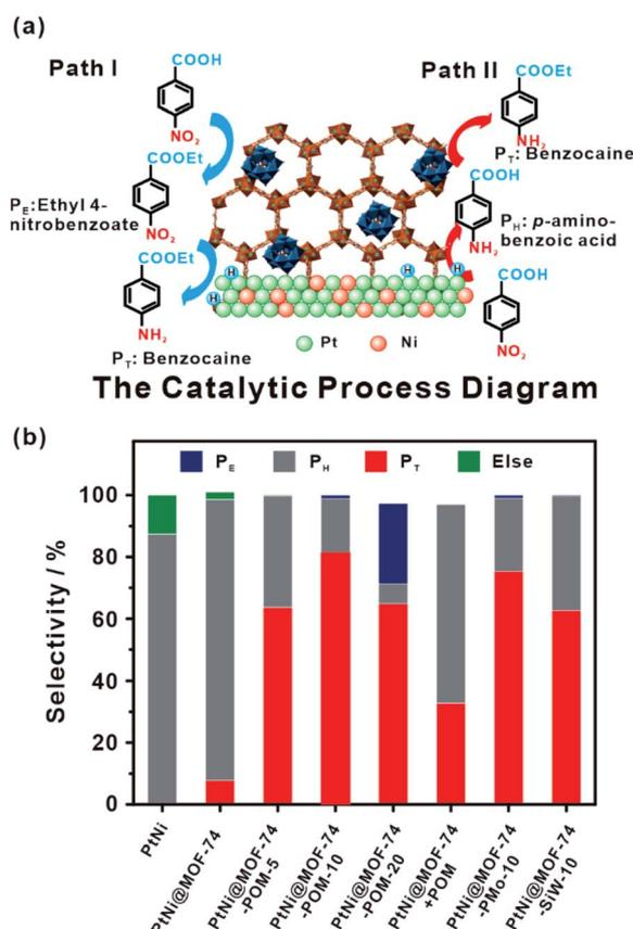
Fig. 20 (a) Schematic illustration of tandem catalytic mechanism on PtNi@MOF-74-POM. (b) Catalysis of tandem reaction with different catalysts. Reproduced with permission.<sup>189</sup> Copyright©2019 The Royal Society of Chemistry.
