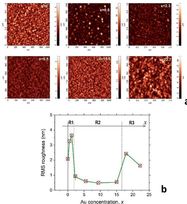
**Fig. 2** (a) AFM images of the surface morphology of selected  $Au_xC_{60}$  films. The Au concentrations  $x$  in the films were added to the respective images. (b) Variation of the RMS surface roughness of the  $Au_xC_{60}$  films with increasing  $x$ . R1, R2 and R3 indicate three different  $x$  intervals in which the  $Au_xC_{60}$  nanostructures possess a common structural feature. Vertical dashed lines indicate the border (critical points,  $x_c$ ) between the intervals (see text).
