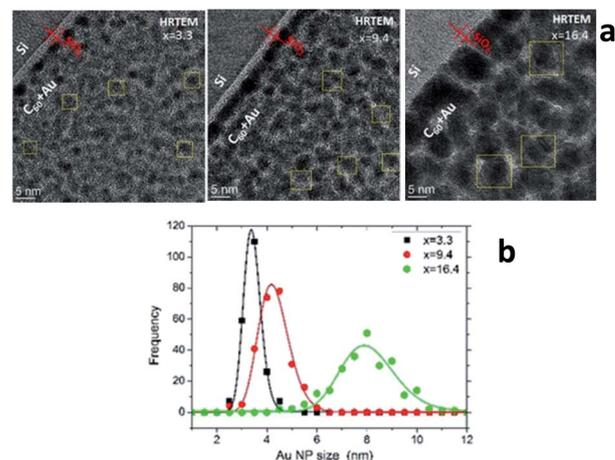
**Fig. 4** (a) HRTEM images of samples S2, S5 and S8. The whitish strip between the Si substrate and  $\text{Au}_x\text{C}_{60}$  mixture film corresponds to native  $\text{SiO}_2$  layer (about 2 nm in thickness). (b) Log-normal size distribution of the Au NPs in samples S2, S5 and S8 as obtained from the analysis of approximately 250 NPs per sample.
