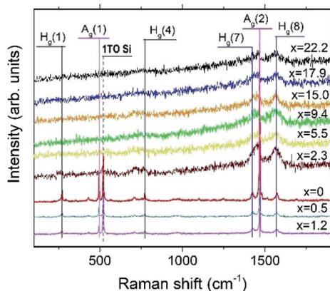
Fig. 9 Raman spectra of the  $\text{Au}_x\text{C}_{60}$  films with different Au concentrations ( $x$ ). The  $x$  values are shown for the respective spectra. Some of the  $\text{C}_{60}$  vibration modes with  $\text{A}_g$  and  $\text{H}_g$  symmetry are indicated by vertical lines. The position of the intense 1TO Si(100) mode is indicated by the dashed vertical line (see text).
