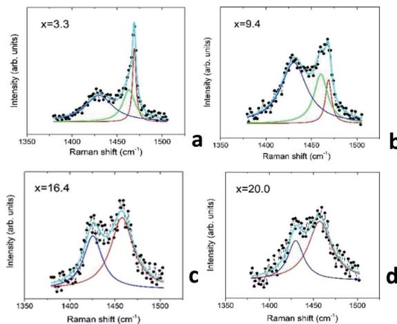
Fig. 10 Raman spectra of the  $\text{Au}_x\text{C}_{60}$  mixture films near the positions of the  $\text{H}_g(7)$  and  $\text{A}_g(2)$  modes of  $\text{C}_{60}$ : (a and b) the mixture films from the interval R2; (c and d) the mixture films from the interval R3. The experimental spectra (black dots) fitted by a superposition of Lorentzians (light-blue line). See description in the text.
